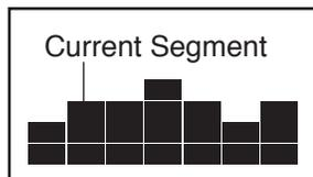
will begin to flash. If a new speed and/or incline setting is programmed for the next segment, the new speed and/or incline setting will appear in the displays. The treadmill will then automatically adjust to the new speed and/or incline setting.
