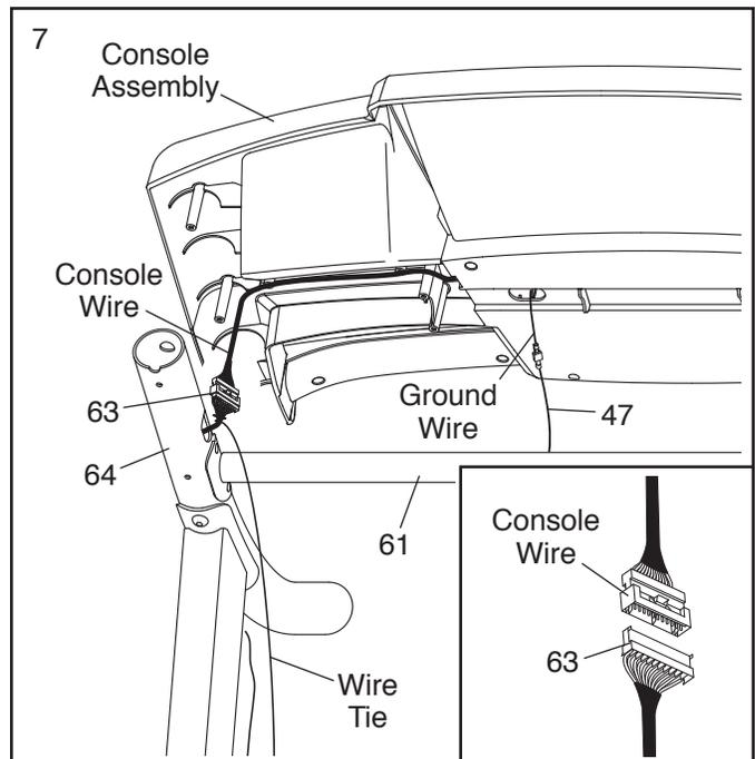
8. Insert the wires into the Right Handrail (64) through the indicated hole as you set the console assembly on the Left and Right Handrails (59, 64). **Make sure that no wires are pinched.**
