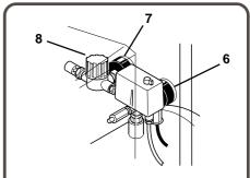
**8) PRESSURE REGULATOR:** The air pressure coming from the air tank is controlled by the regulator knob. Turn the pressure regulation knob clockwise to increase discharge pressure, and counterclockwise to decrease discharge pressure.
