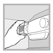
Access the light bulb by removing the cover as indicated in the diagram. Replace it with a similar light bulb within the power range indicated on the cover (10W or 15W).
