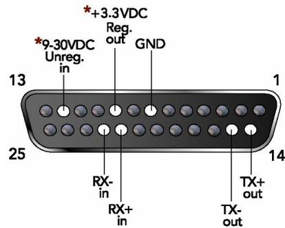
**DB25 Female DCE Interface RS485/422***\*Optional power connection*
