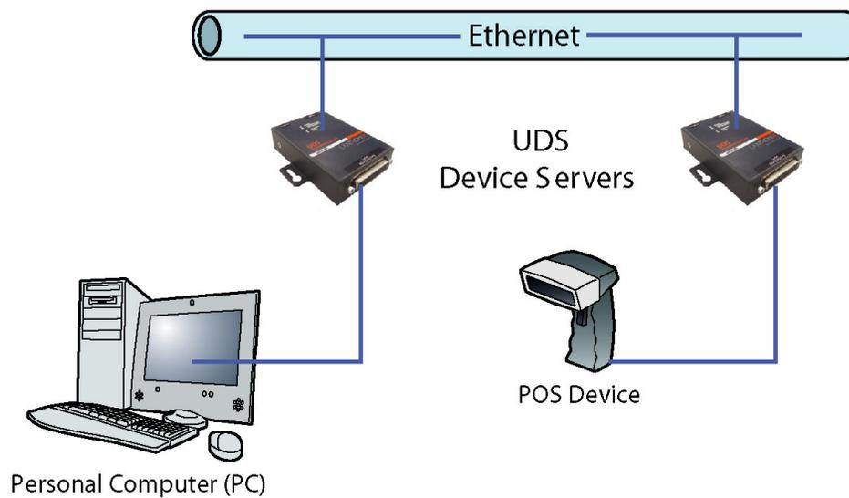
The Com Port Redirector software included on the product CD simplifies the integration process by extending the functionality of COM-port-based Windows™ applications. Virtual COM ports, mapped to remote device servers on the network, can replace direct serial connections.
