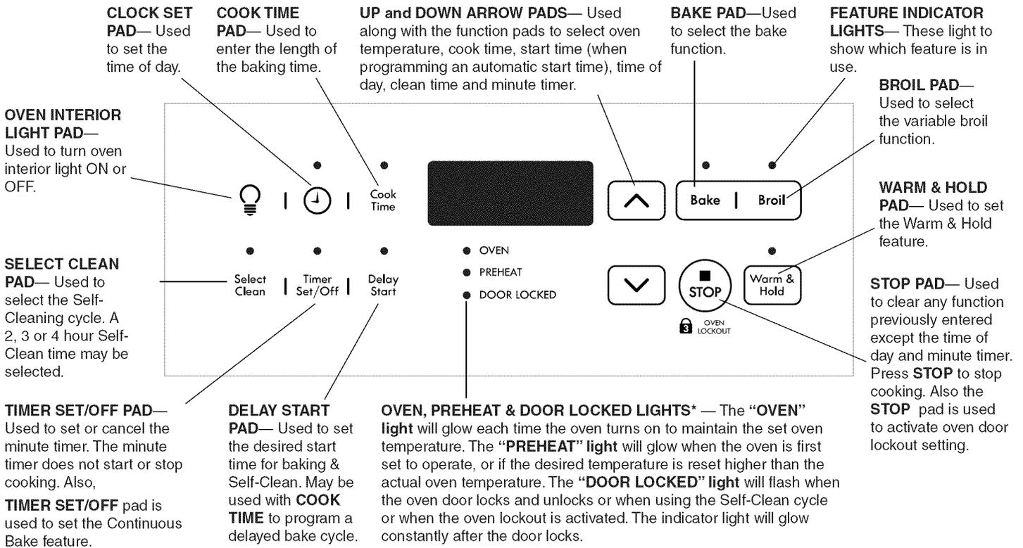
\*Note: The **OVEN** indicator light on the electronic display will turn ON and OFF when using the Bake feature and during preheat. This is normal and indicates that the oven is cycling to maintain the selected baking temperature. When the pre-heat indicator light turns OFF, your oven has reached the set temperature.
