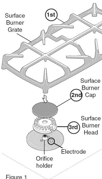
**To Remove and Replace the Surface Burner Caps and Burner Heads -** Remove in the following order: (1st) surface Burner Grates, (2nd) Burner Caps and (3rd) Burner Heads. Replace them in reverse order: Heads, Caps, then Grates.
