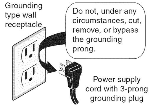
**⚠ WARNING** Avoid fire hazard or electrical shock. **DO NOT** use an adapter plug, an extension cord, or remove grounding prong from electrical power cord. Failure to follow this warning can cause serious injury, fire or death.
