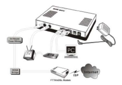
The figure above shows how to connect an xDSL modem to a home coaxial cable network. Follow the same steps to connect any Ethernet device such as a HUB or printer, to a coaxial cable network. Now you should have connected the **LAN** port, **HCNA** port and the **DC5V** port to the appropriate devices or lines. LED will be as:
