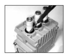
9. If the crankcase oil seals (19) are to be replaced, they can be removed by prying loose with a flat screwdriver. Take care not to make contact with the plunger.
