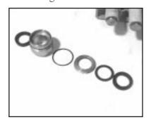
7. Remove the weep return ring (25), pressure ring (24), and v-sleeve (23) from the valve casing (26). Remove the v-sleeve (23) from the seal case (20).
