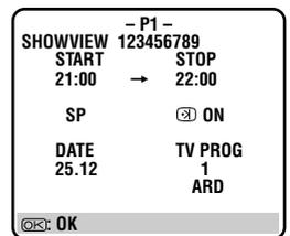
The display panel shows the programme start time. Pressing **PROG CHECK** changes the display to the programme stop time, then the date and channel position.
