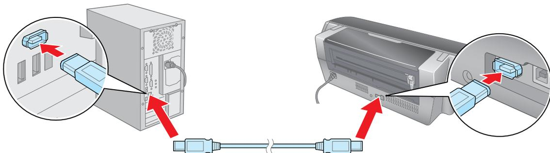
**NOTE:** If your computer uses i.Link or another 4-pin FireWire connection, you will need to connect a 6-pin to 4-pin FireWire (IEEE 1394) cable.
