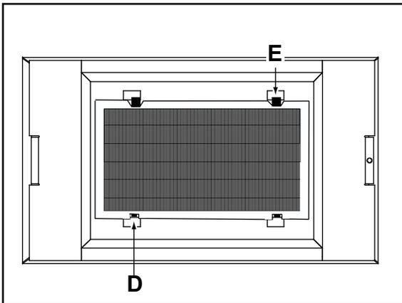
Install charcoal filter (plastic side up) into filter bracket. Insert tab cut-out side **D** of charcoal filter into bracket first. Lock charcoal filter into place by pushing down on side **E** with locking tabs.
