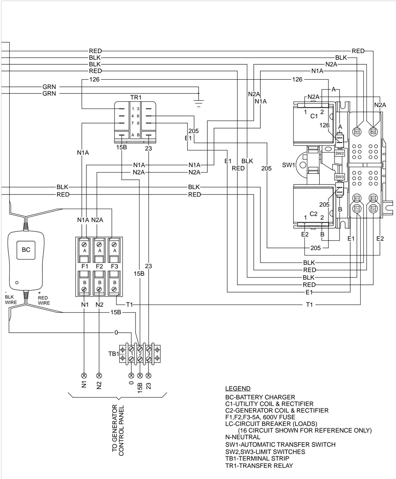
Figure 2. Wiring Diagram
