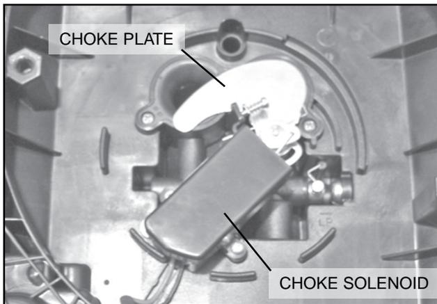
Figure 22. Solenoid De-Energized, Choke Closed
