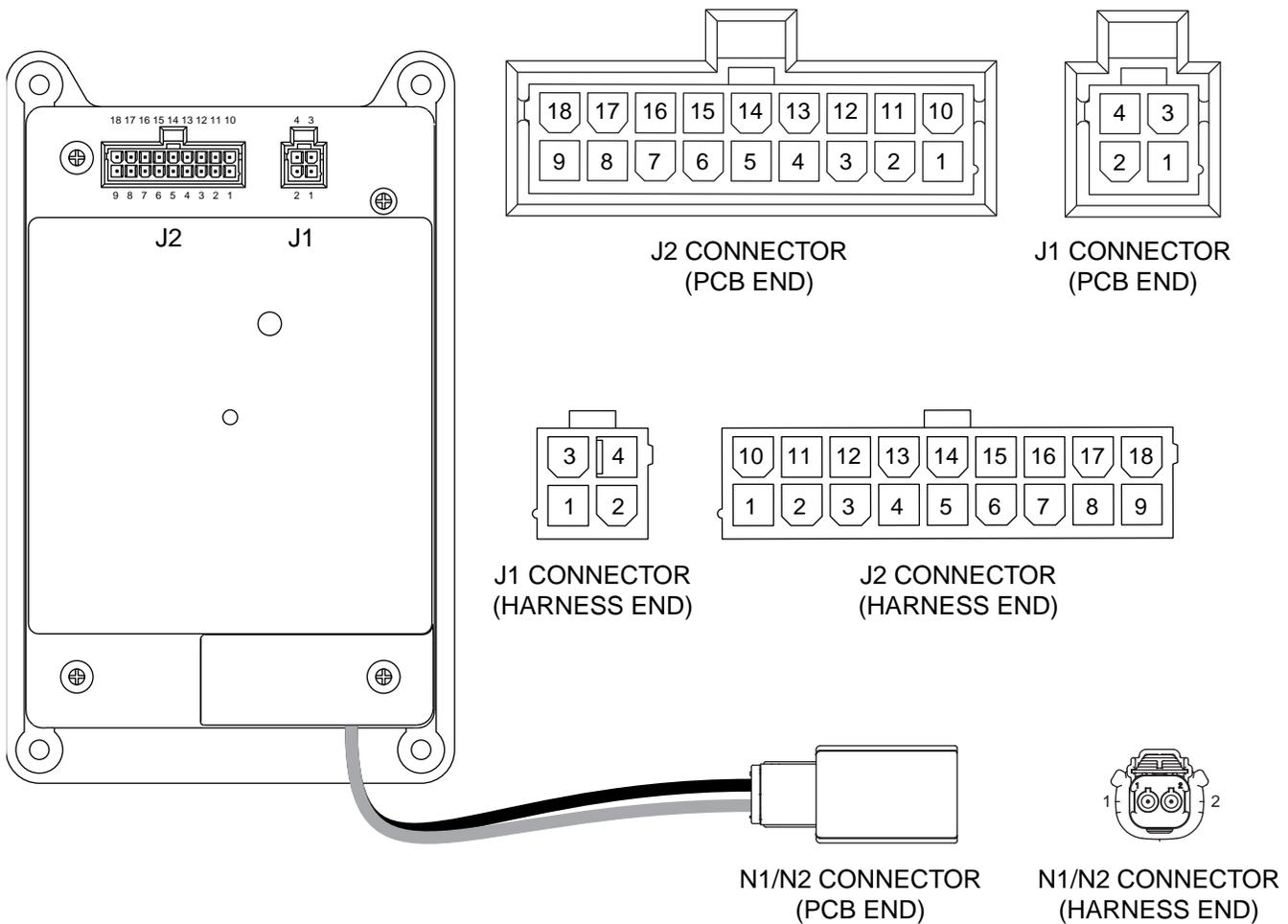
Figure 4. 8 kW Printed Circuit Boards and J1 Connector
