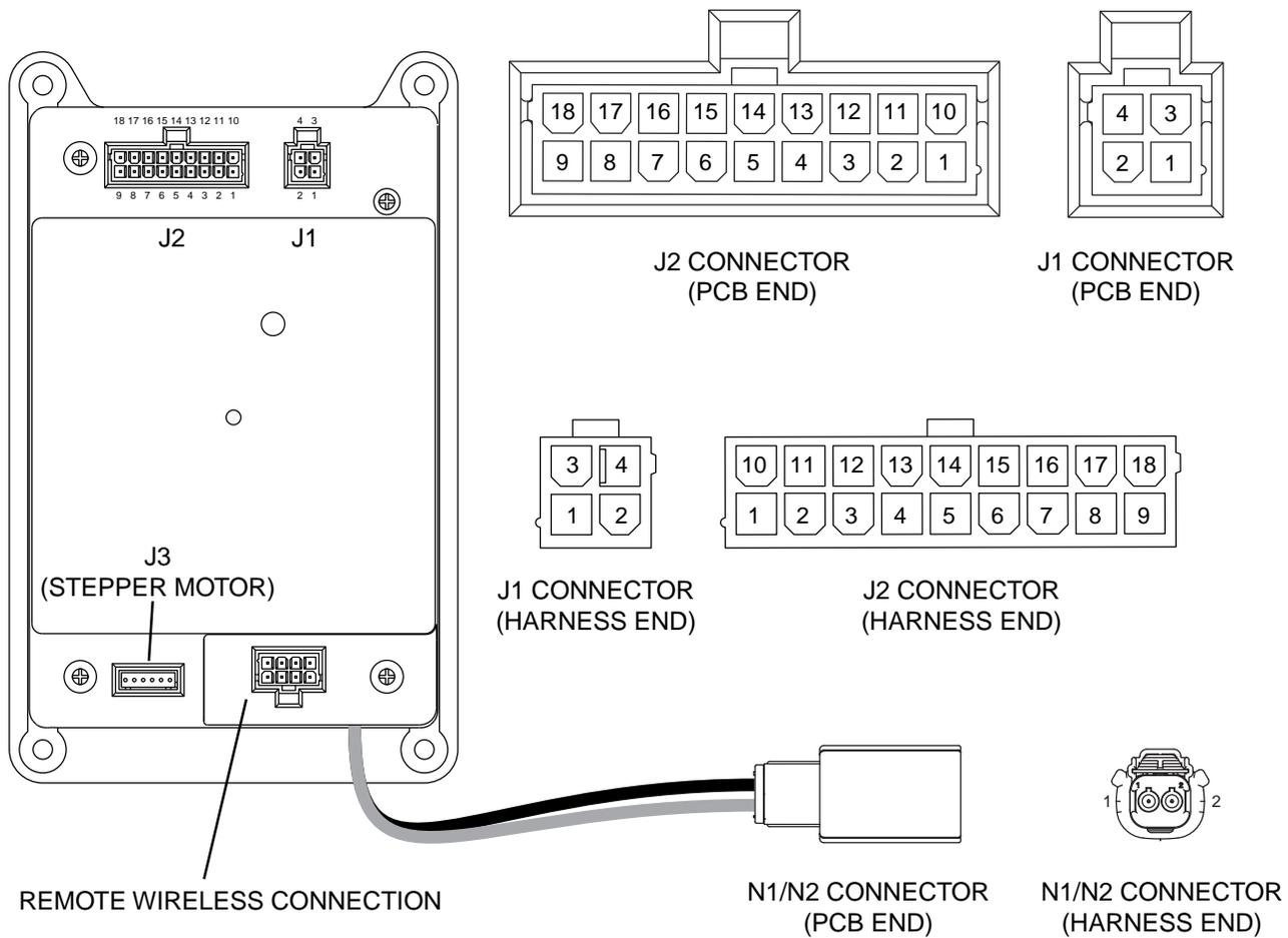
Figure 6. 12/14 kW Printed Circuit Board and J1 Connector
