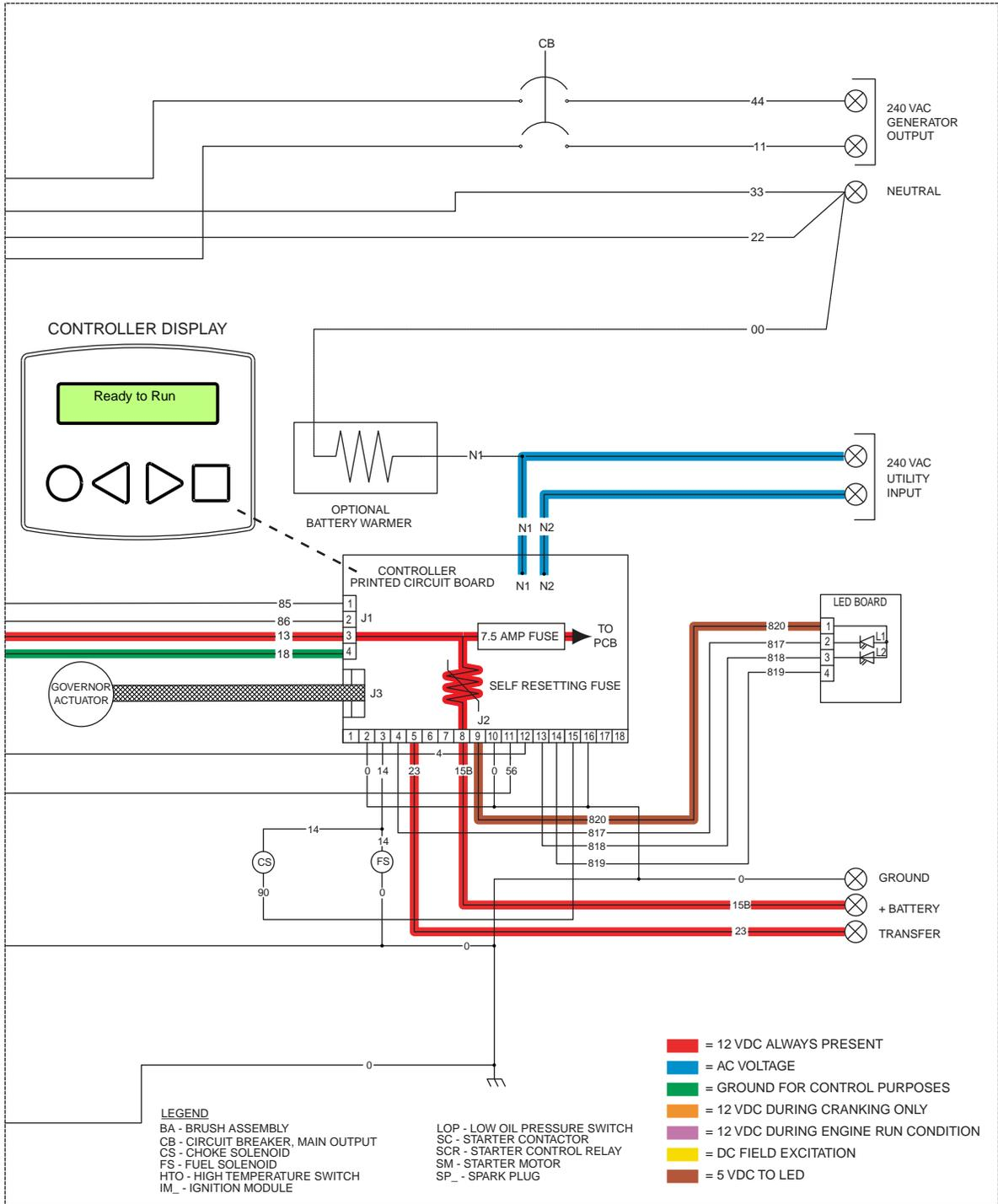
**INITIAL DROPOUT OF UTILITY SOURCE VOLTAGE**
