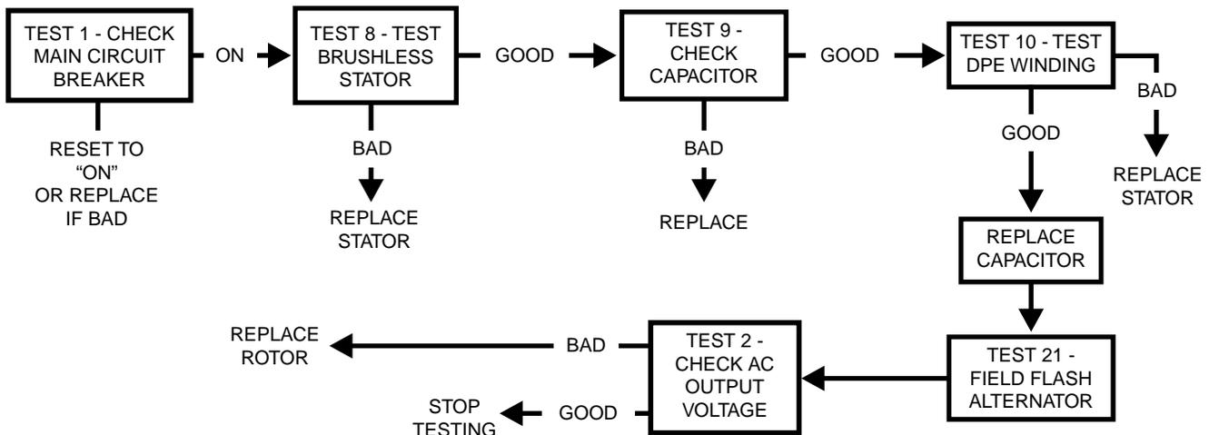
**Problem 3 - Generator Produces Low Voltage at No-Load**
