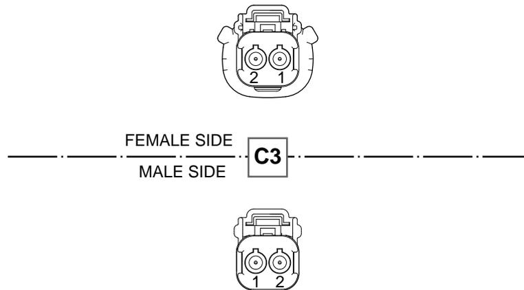
Figure 8. Choke Solenoid Connector Pin Number Identification
