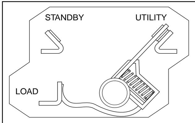
Figure 2. Load Connected to Utility Power Source
