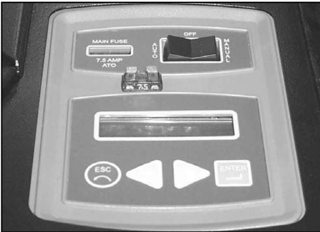
*Figure 1. Remove 7.5 Amp Fuse*
