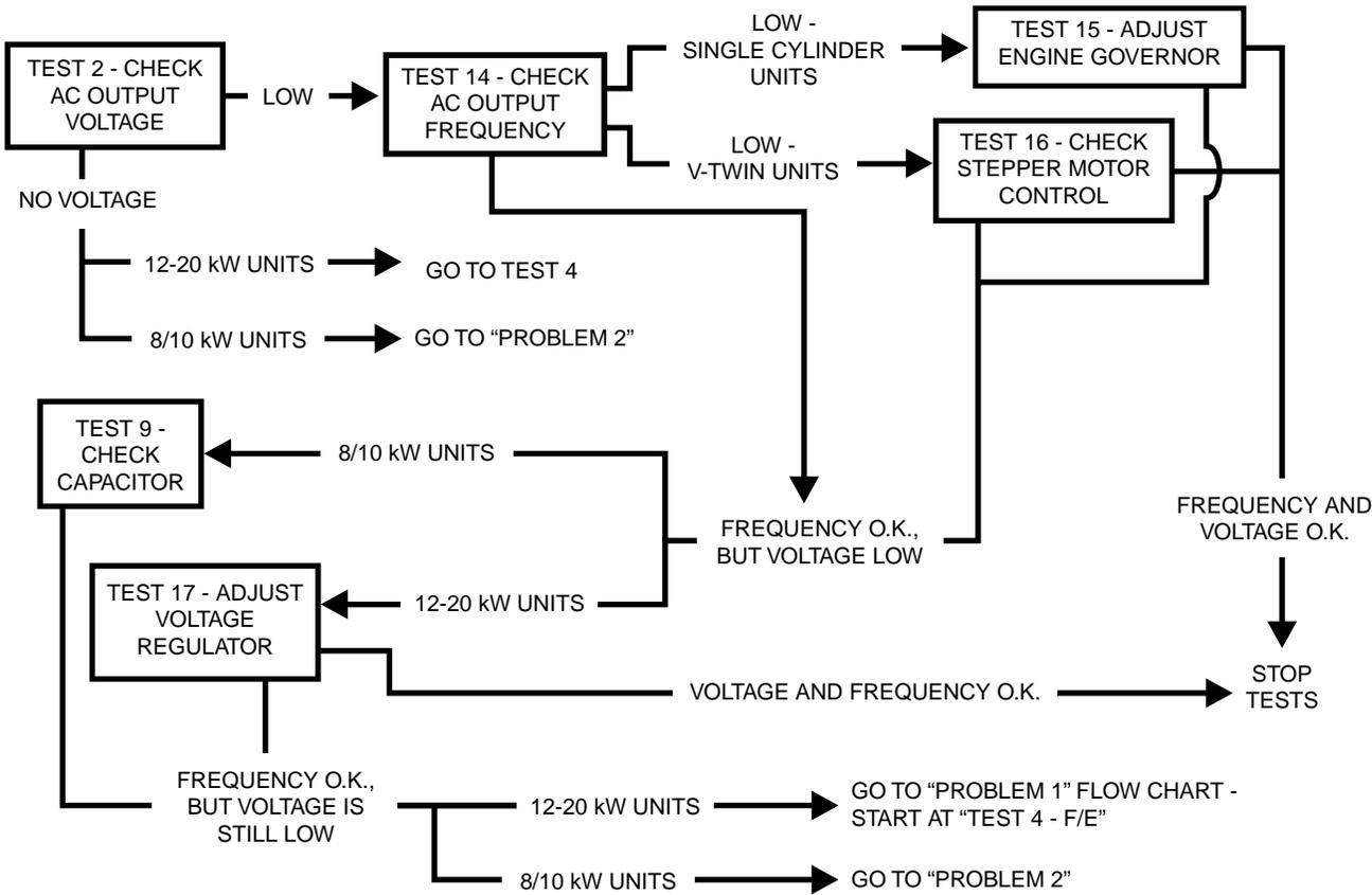
**Problem 4 - Generator Produces High Voltage at No-Load**
