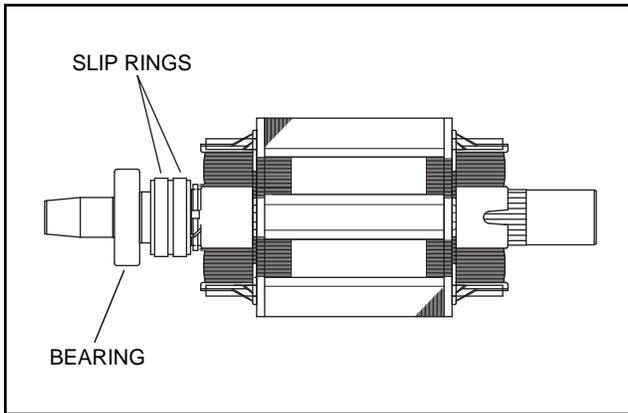
Figure 2. The 2-Pole Rotor Assembly 12-20 kW
