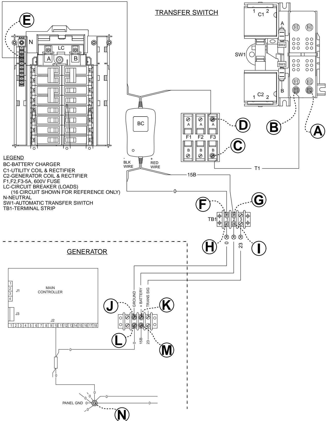
Figure 11. Test 40, 41, and 42 "Pre-Wire Load Center" Test Points.
