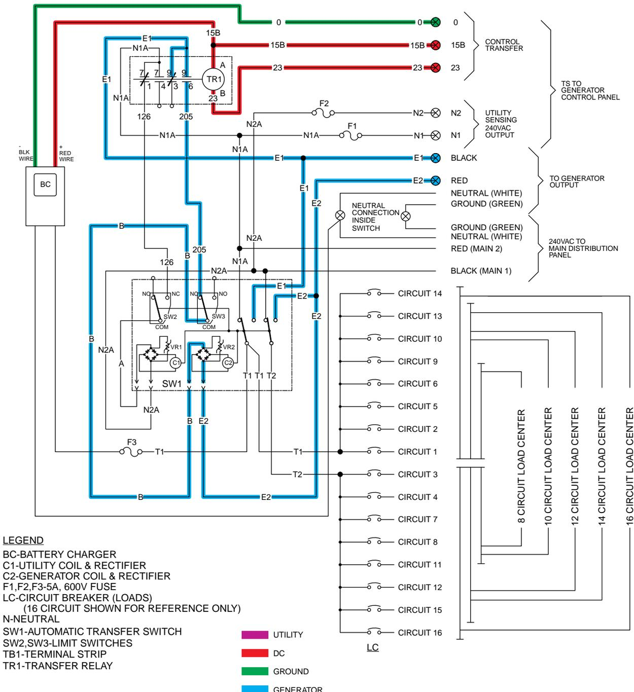
Figure 4. Generator Power Available, Waiting to Transfer.
