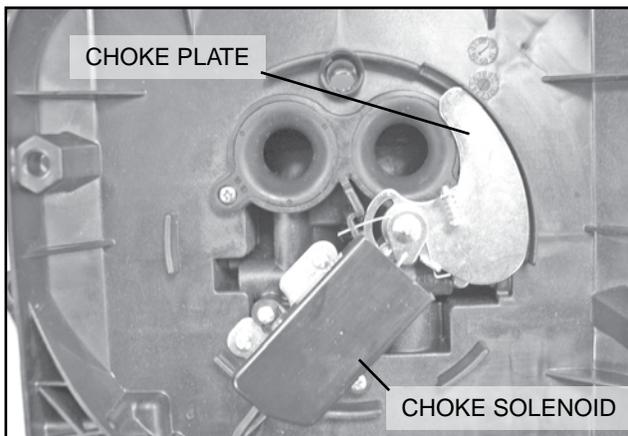
Figure 23. Solenoid Energized, Choke Open
