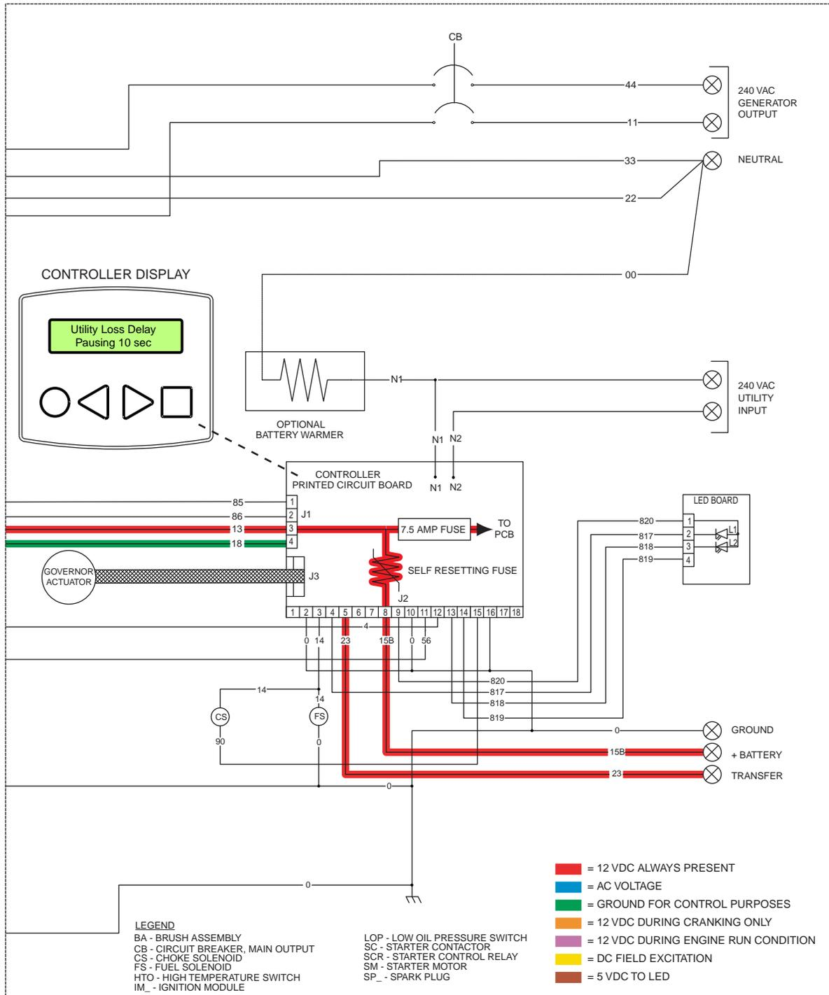
**UTILITY VOLTAGE DROPOUT AND ENGINE CRANKING**
