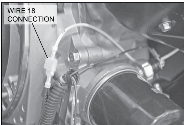
Figure 33. Wire 18 Connection 8 kW Units
