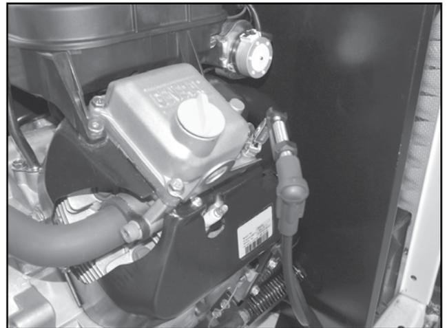
Figure 28. Checking Ignition Spark
