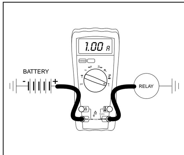
Figure 4. A VOM as an In-line meter
