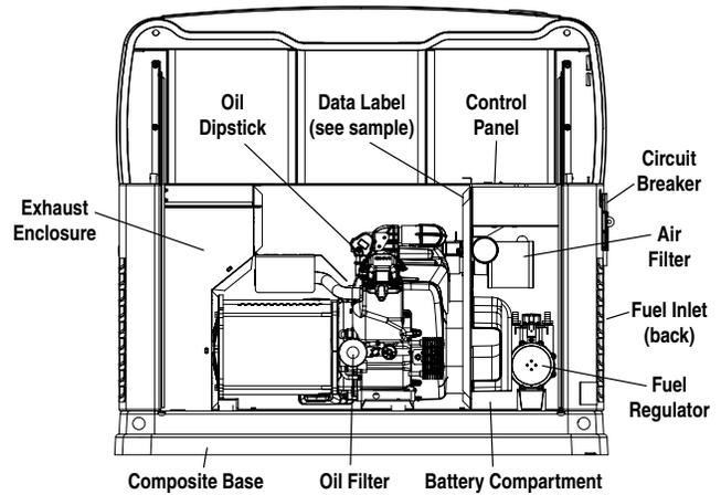
Figure 1.3 – 12, 14, 16, 17 and 20kW, V-twin,
