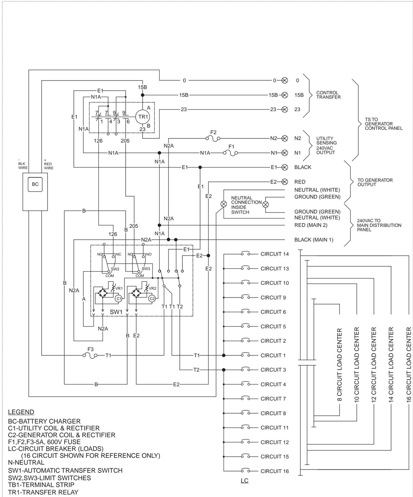
Figure 1. Schematic
