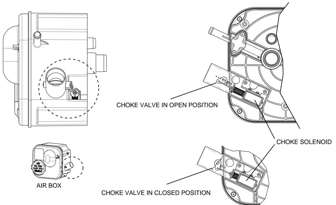
Figure 26. 8kW Choke Solenoid
