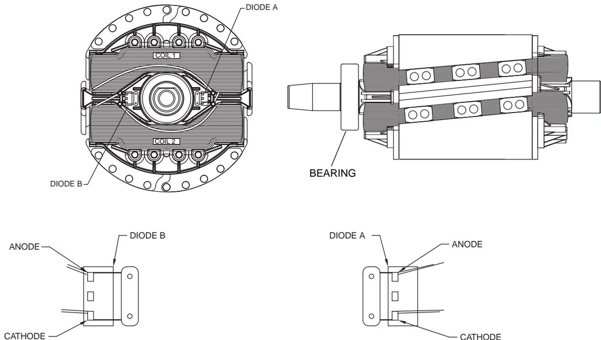
Figure 3. The 2-Pole Rotor Assembly 8/10kW
