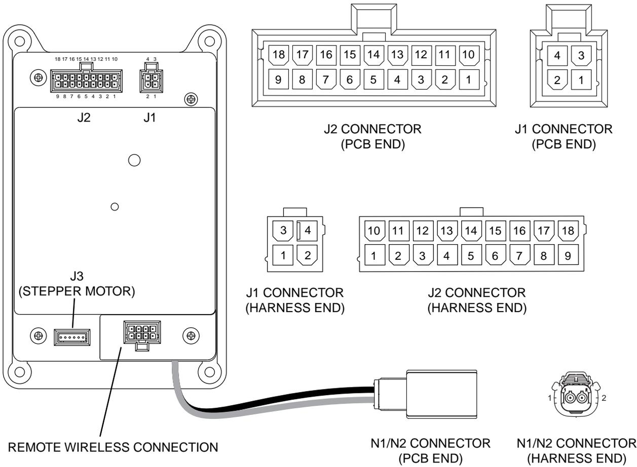
*Figure 5. 10 kW Printed Circuit Board and J1 Connector*
