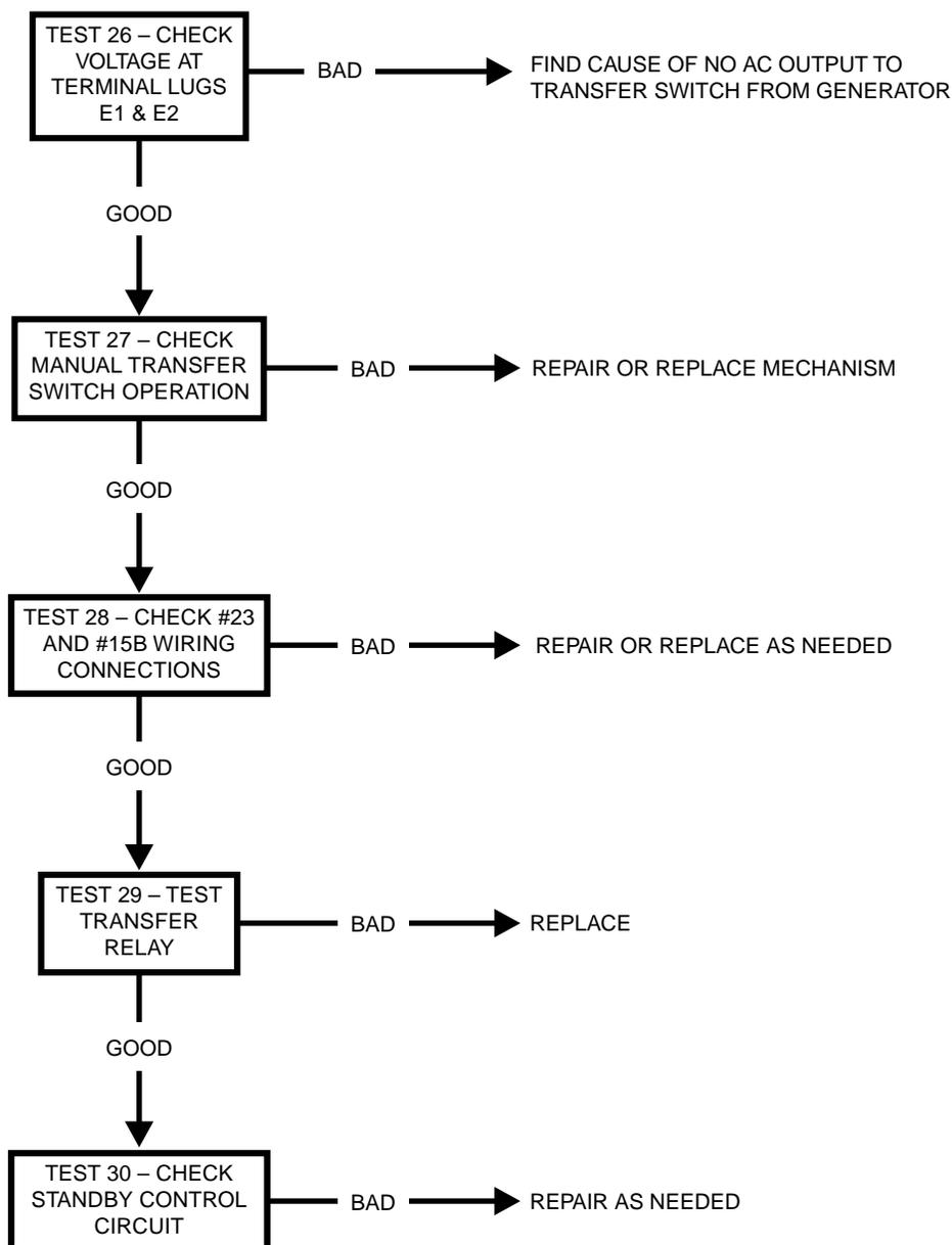
***Problem 8 – In Automatic Mode, Generator Starts When Loss of Utility Occurs, Generator Shuts Down When Utility Returns But There Is No Retransfer To Utility Power
