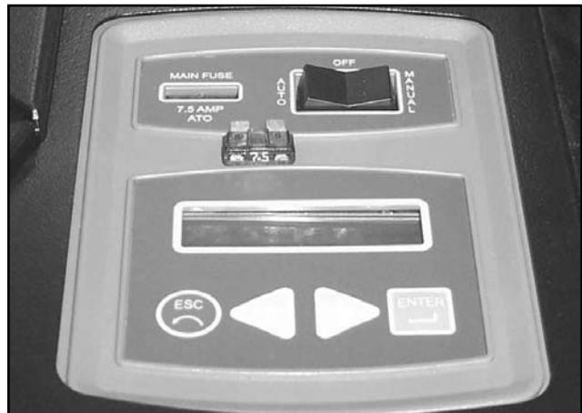
Figure 22. Remove 7.5 Amp Fuse
