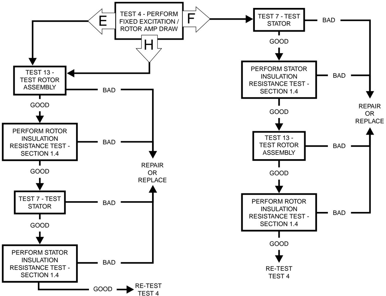
**Problem 2 - Generator Produces Zero Voltage or Residual Voltage
