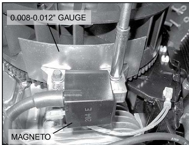
Figure 34. Setting Ignition Magneto (Armature) Air Gap
