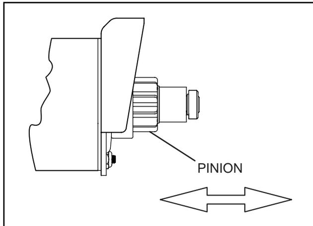
Figure 13. Check Pinion Gear Operation
