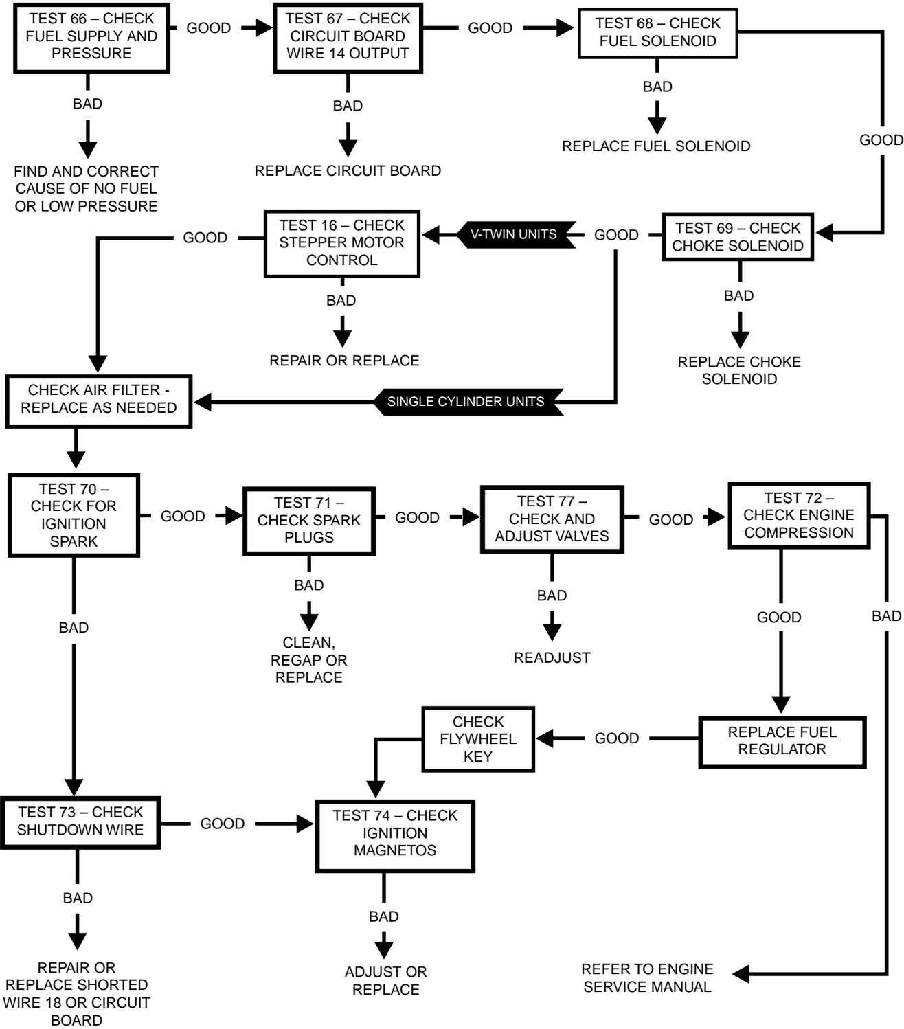
***Problem 18 – Engine Starts Hard and Runs Rough / Lacks Power / Backfires***
