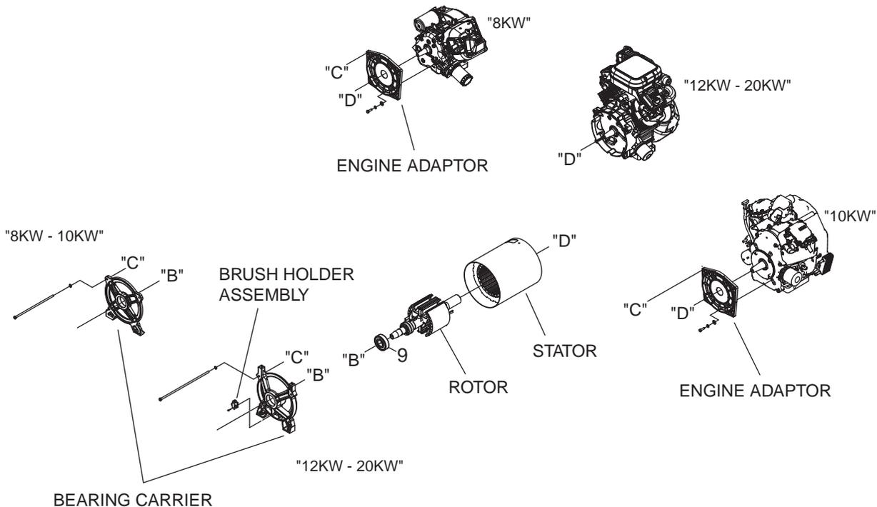
Figure 1. AC Generator Exploded View
