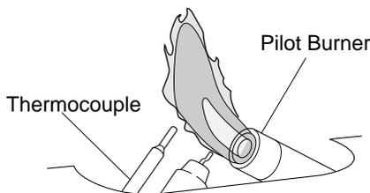
Figure 18 - Incorrect Pilot Flame Pattern
