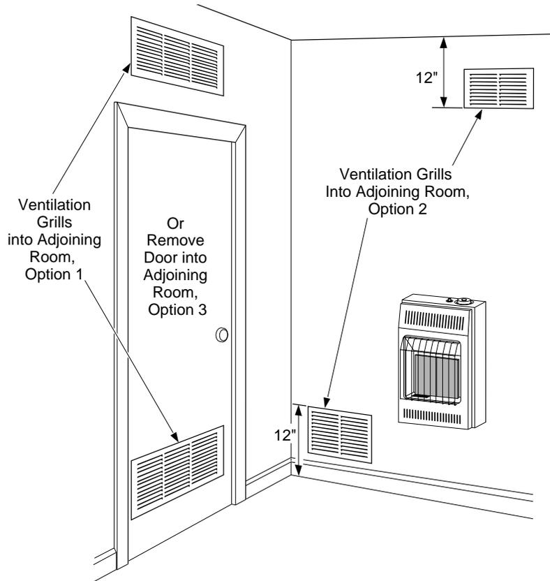
Figure 2 - Ventilation Air from Inside Building
