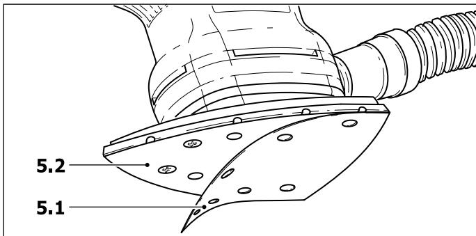
The self-adhesive sanding material (5.1) is simply pressed onto the sanding base (5.2) and held safely in place by the Stickfix sanding base velcro surface.
