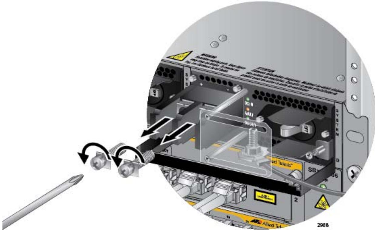
Figure 117. Removing the Terminal Screws
