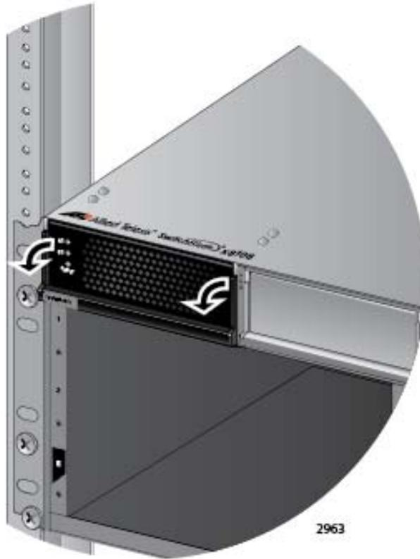
Figure 58. Locking the Handle on the AT-SBxPWRPOE1 Power Supply
