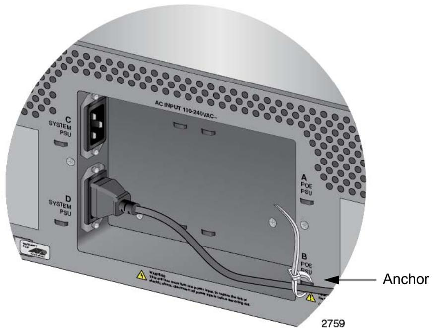
Figure 99. Securing the Power Cord for the AT-SBxPWRSYS1 AC Power Supply to an Anchor
