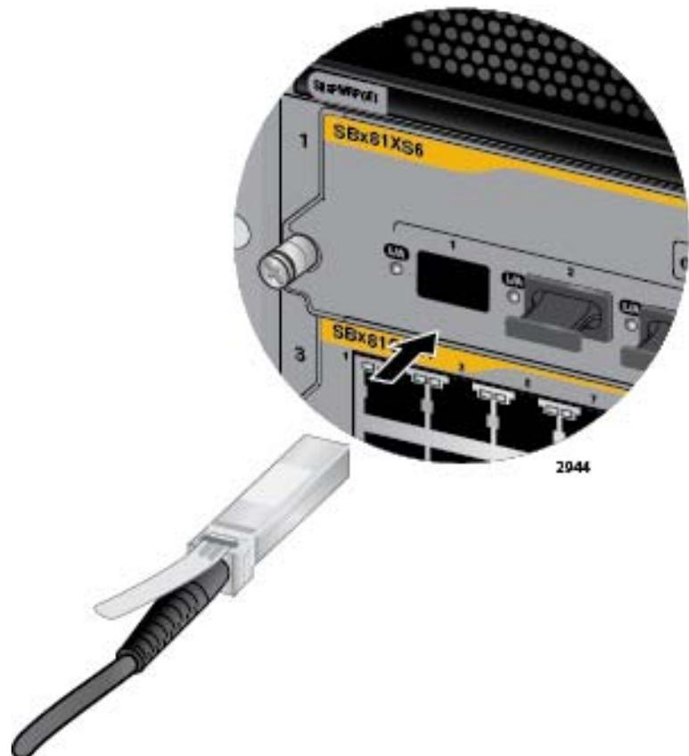
Figure 96. Installing the AT-SP10TW Cable in the AT-SBx81XS6 Line Card
