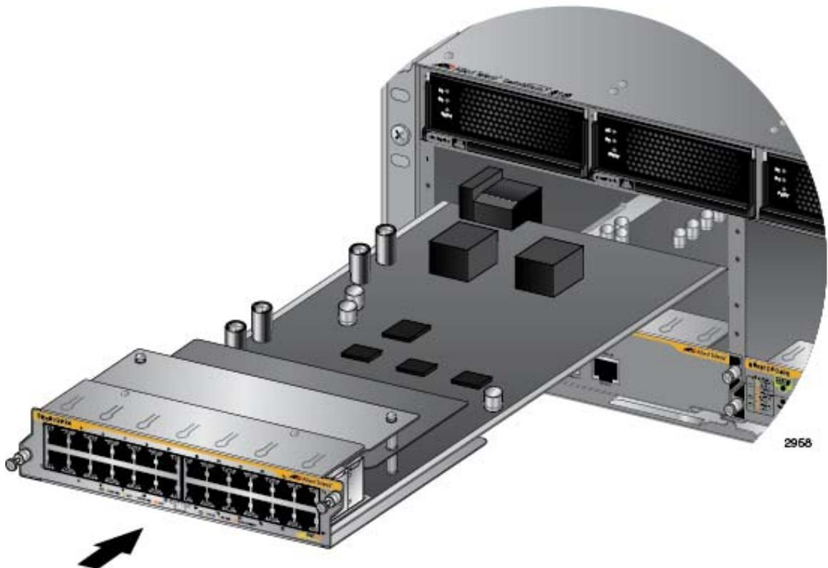
Figure 75. Aligning an Ethernet Line Card in a Chassis Slot
