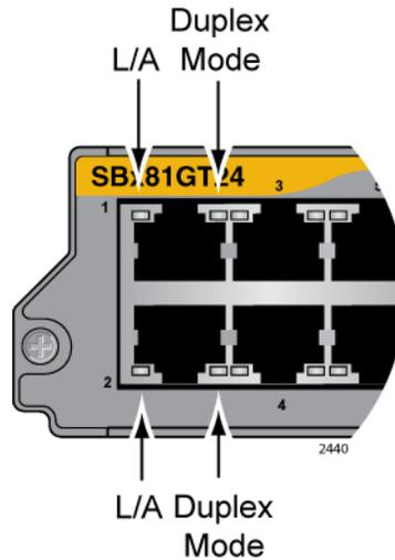
Figure 16. Port LEDs on the AT-SBx81GT24 Line Card
