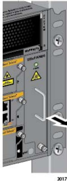
Figure 154. Loosening the AT-SBxFAN06 Fan Module from the Backplane Connector
