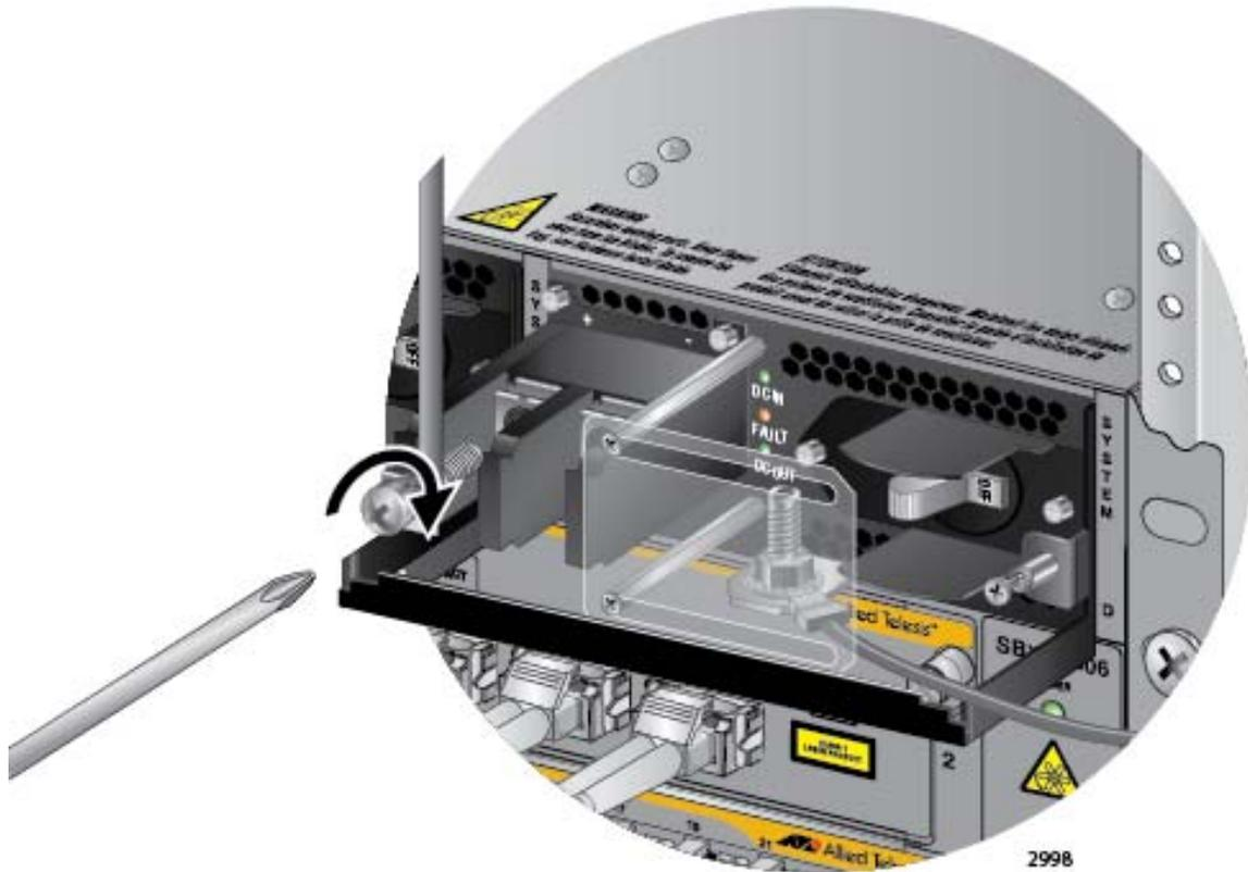
Figure 130. Connecting the Positive Lead Wire
