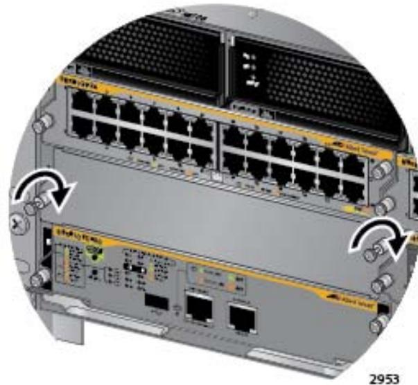
Figure 79. Tightening the Thumbscrews on a Blank Slot Cover
