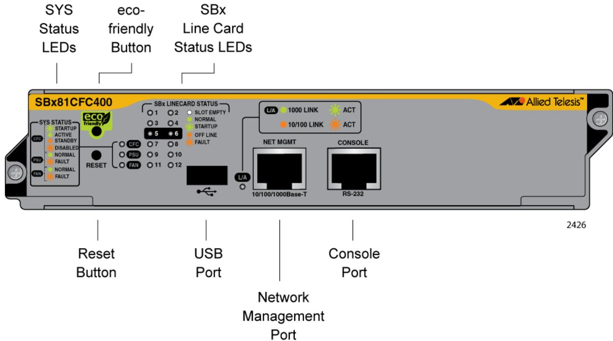
Figure 22. AT-SBx81CFC400 Controller Fabric Card
