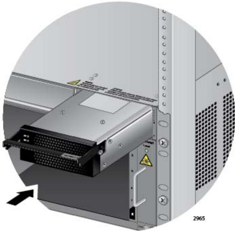
Figure 51. Inserting the AT-SBxPWRSYS1 Power Supply
