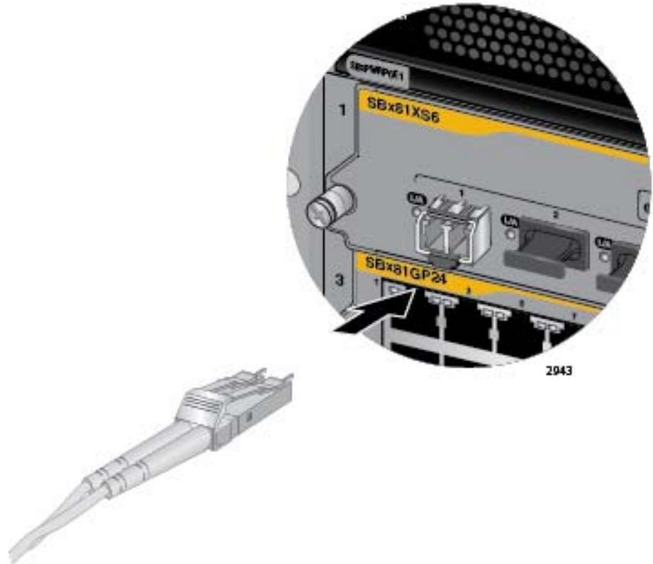
Figure 93. Attaching a Fiber Optic Cable to an SFP+ Transceiver in the AT-SBx81XS6 Line Card
