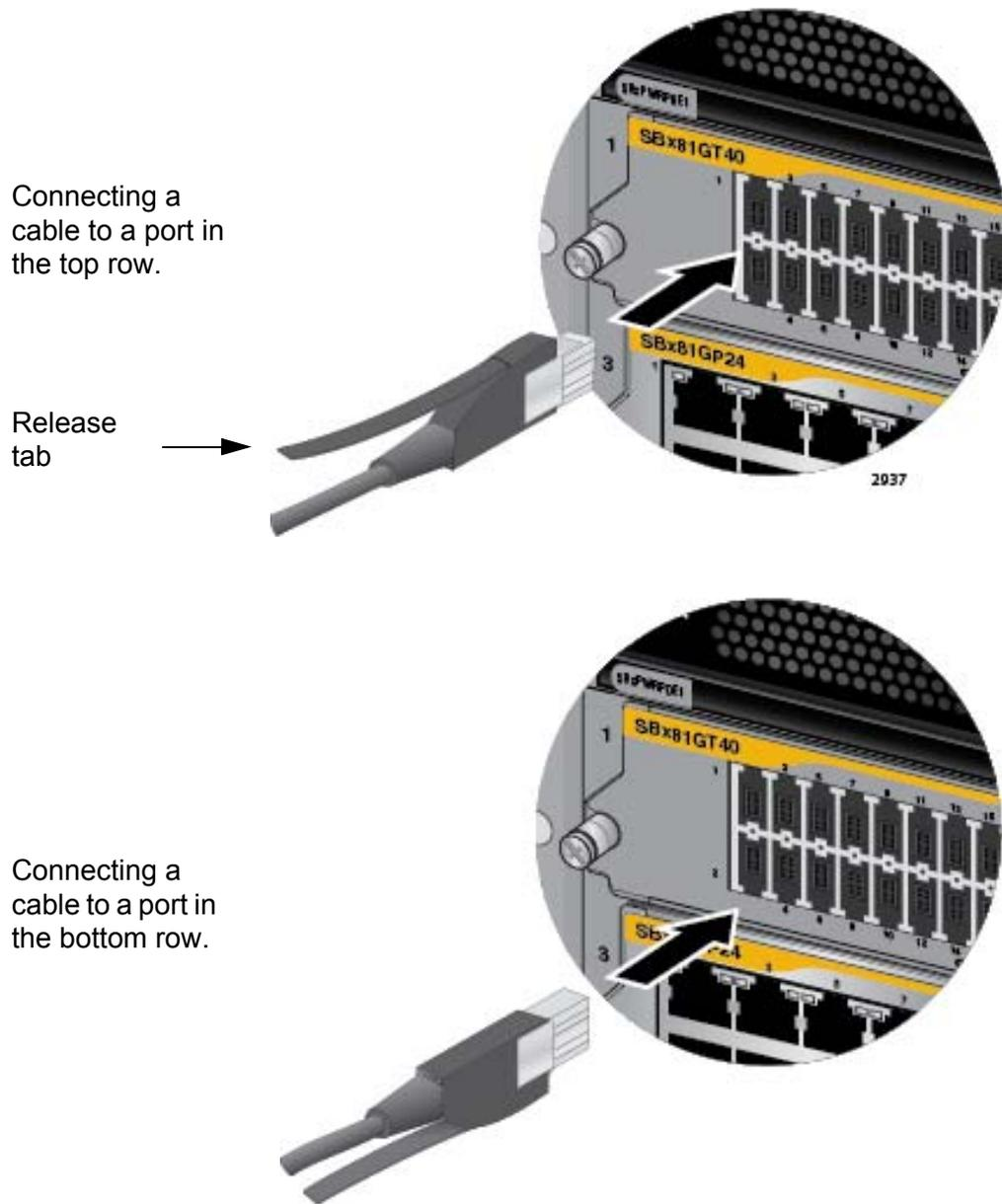
Figure 81. Connecting Cables to Ports on the AT-SBx81GT40 Line Card
