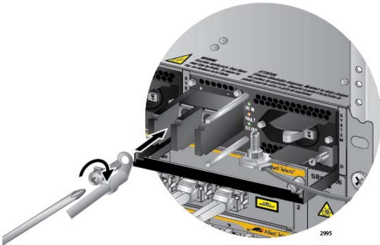
Figure 126. Connecting the Positive (+) Power Wire with a Right Angle Terminal
