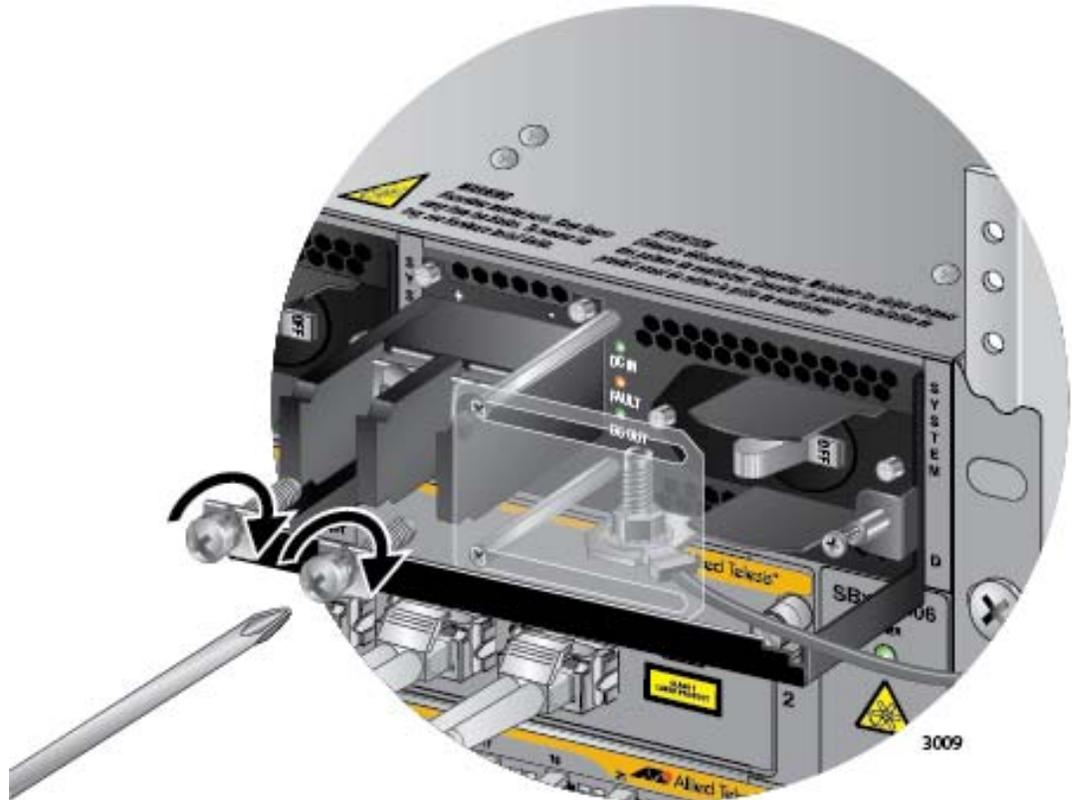
Figure 146. Reinstalling the Screws on the Positive and Negative Terminals
