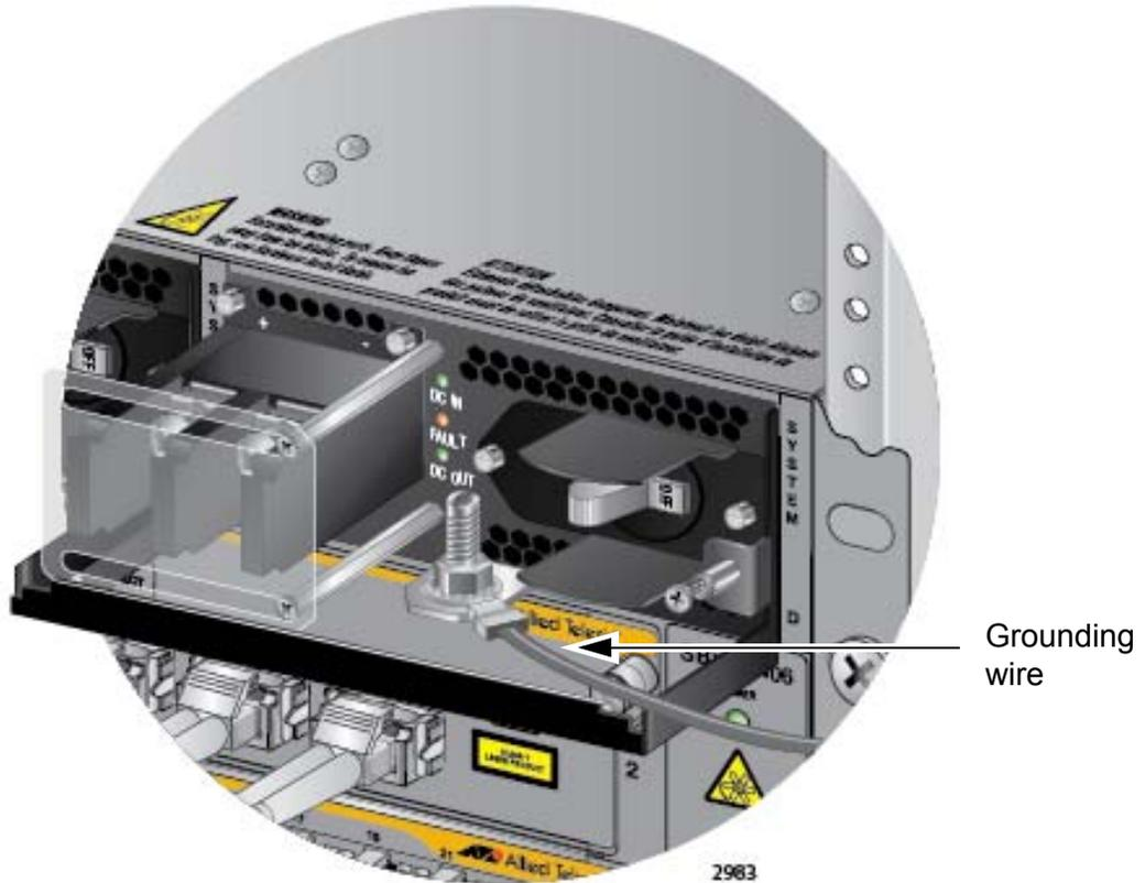
Figure 108. Installing the Grounding Wire
