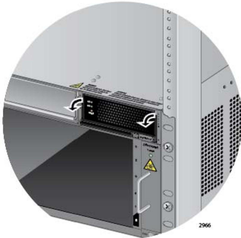
Figure 52. Lowering the Handle on the AT-SBxPWRSYS1 Power Supply
