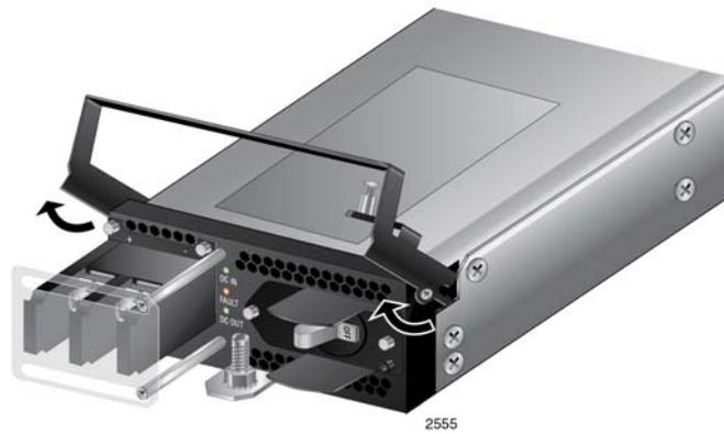
Figure 62. Raising the Handle on the AT-SBxPWRPOE1 DC Power Supply
