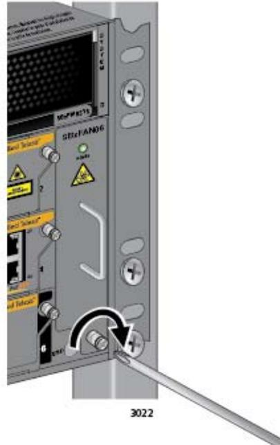
Figure 159. Tightening the Screw on the AT-SBxFAN06 Fan Module
