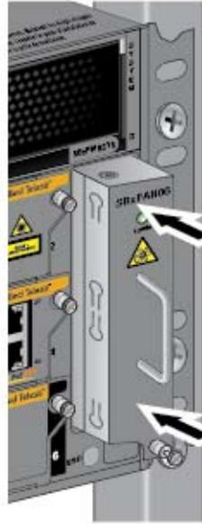
Figure 158. Securing the AT-SBxFAN06 Fan Module on the Backplane Connector
