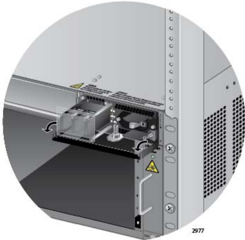
Figure 64. Locking the Handle on the AT-SBxPWRSYS1 Power Supply
