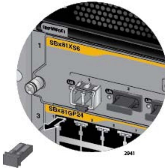
Figure 91. Removing the Dust Cover from an SFP+ Transceiver in the AT-SBx81XS6 Line Card
