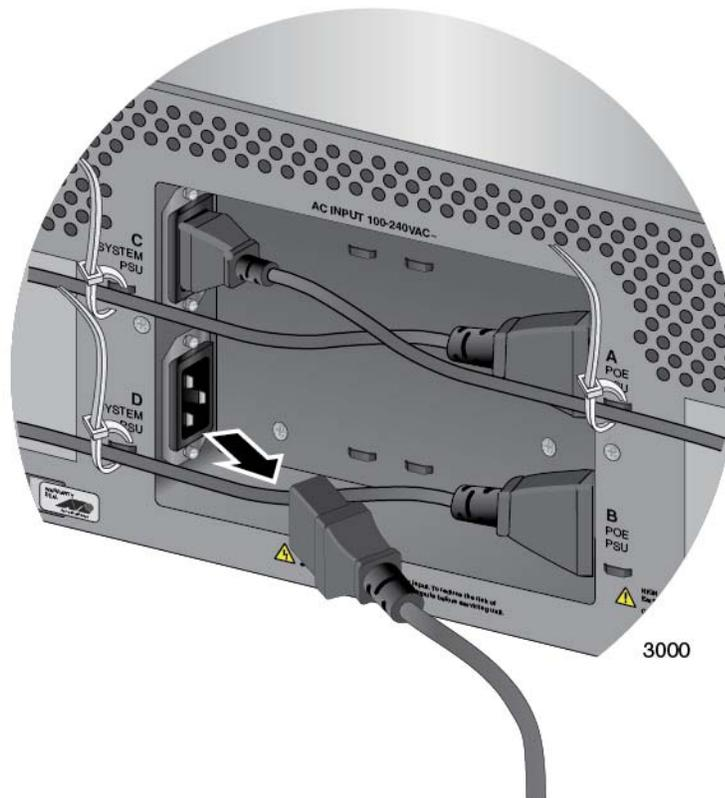
Figure 137. Disconnecting the AC Power Cord from the AC Socket on the Back Panel
