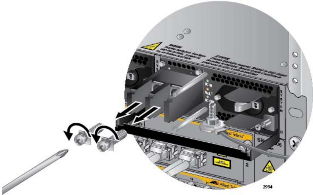
Figure 125. Removing the Terminal Screws
