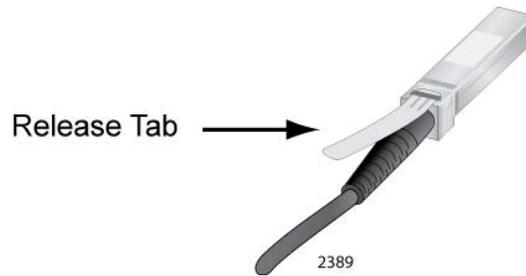
Figure 95. Release Tab on the AT-SBx81XS6 Line Card
