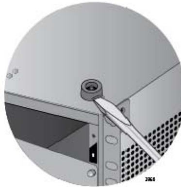
Figure 34. Removing the Rubber Feet
