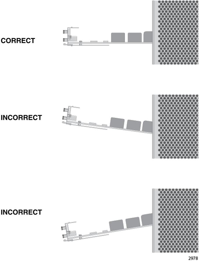
Figure 65. Aligning Card in Slot
