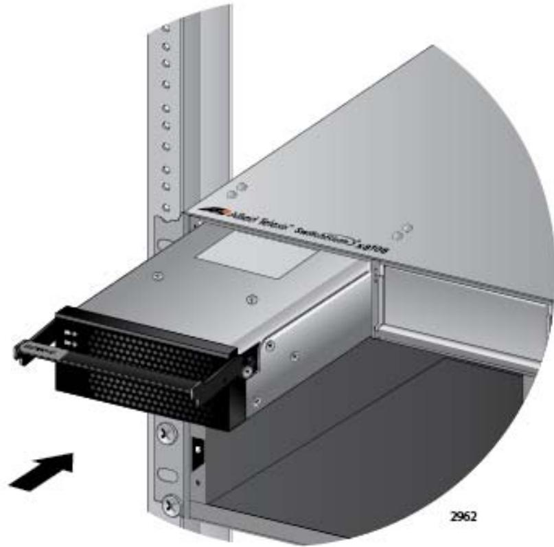
Figure 57. Inserting the AT-SBxPWRPOE1 Power Supply
