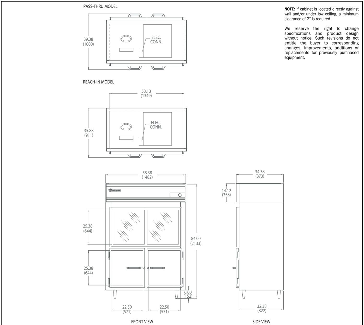
**NOTE:** If cabinet is located directly against wall and/or under low ceiling, a minimum clearance of 2" is required.
