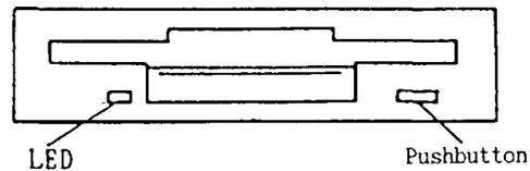
If the main power is turned off and then turned on while the system disk is inserted in the FDD, the controller will be cold started. To prevent this, be sure to turn off the main power after removing the disk from the FDD.
