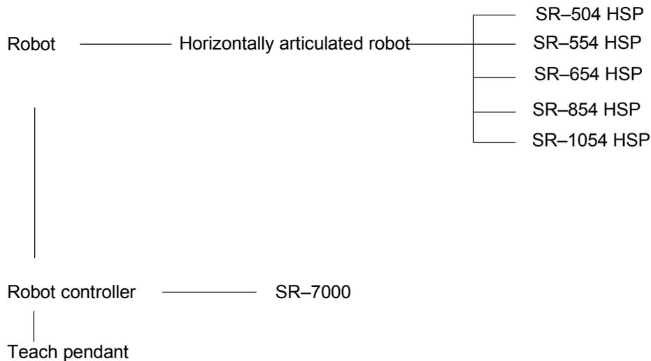
Fig. 1.2 System Configuration of SR Series System Robot
