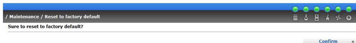
Reset to default value, the password is: **00000000**, and IP address to default DHCP.
