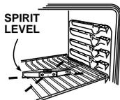
**D7** Remove the storage drawer. The front leveling legs can be accessed from the bottom and the rear legs from the top.
