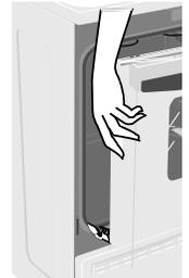
**D10** Place the notch of the hinge arm into the bottom edge of the hinge slot.
