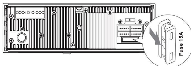
If the fuse gets damaged immediately after it has been replaced, there may be an internal malfunction. In such case, consult your Philips dealer.
