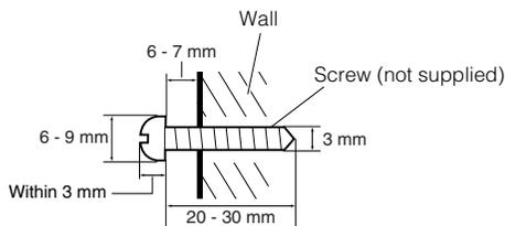
3. Hook the Center Unit onto the attached screws.
