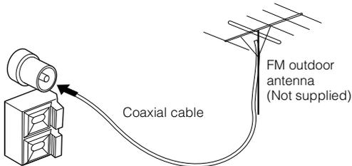
**Using the Coaxial Type Connector (Not Supplied)**
