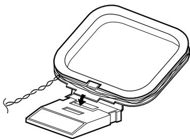
Attach the AM loop to its base by snapping the tabs on the loop into the slot in the base.
