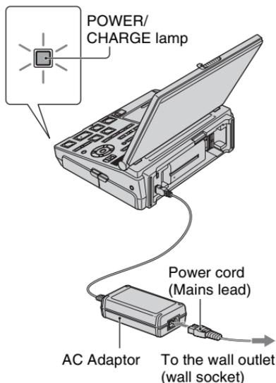
The POWER/CHARGE lamp turns off when the battery pack is fully charged. After charging the battery pack, disconnect the AC Adaptor from the DC IN jack on the VCR.
