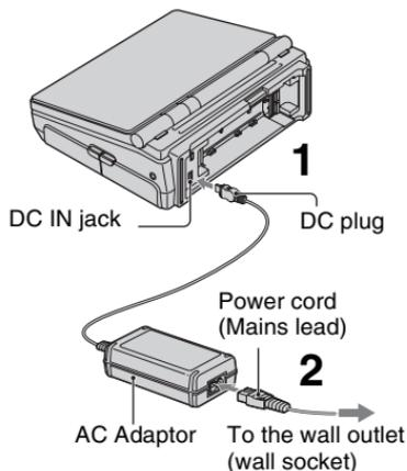
**1** Connect the AC Adaptor to the DC IN jack on the VCR. Make sure that the ▲ mark on the DC plug is facing to the ▲ mark on the VCR.
