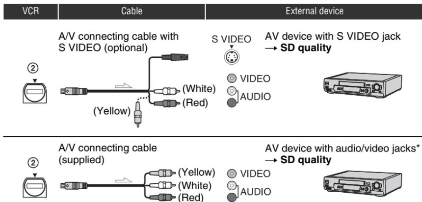
\* When connecting the VCR to a monaural device, connect the yellow plug of the A/V connecting cable to the video jack on the device, then connect the white (left channel) or red (right channel) plug to the audio jack on the device.
