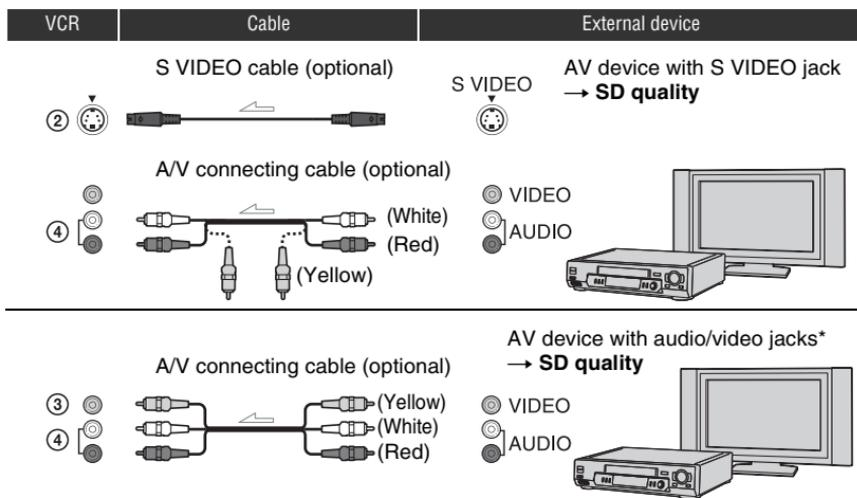
\* When connecting the VCR to a monaural device, connect the yellow plug of the A/V connecting cable to the video jack on the device, and connect the white (left channel) or red (right channel) plug to the audio jack on the device.
