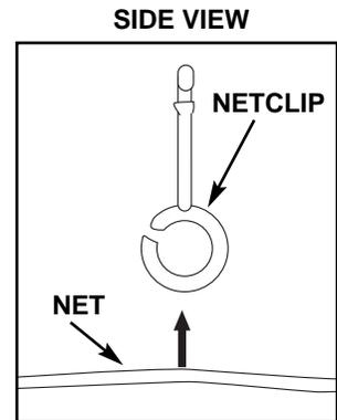
Insert net into bottom of clip as shown.
