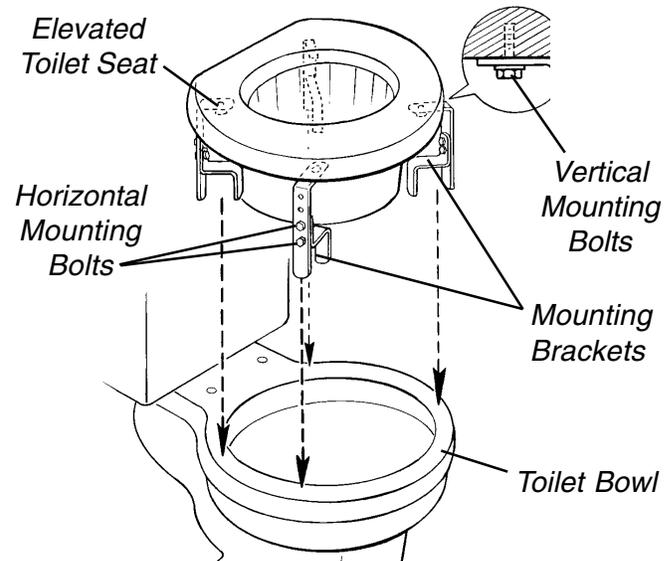
FIGURE 1 - SEAT INSTALLATION/REMOVAL
