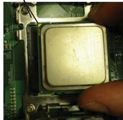
3. Align pin 1 of the CPU with pin 1 of the socket. Once aligned, carefully place the CPU into the socket. *Do not drop the CPU on the socket, move the CPU horizontally or vertically or rub the CPU against the socket or against any pins of the socket, which may damage the CPU and/or the socket.*
