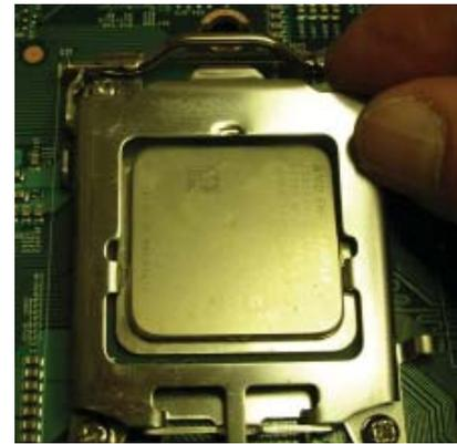
5. Carefully press the CPU socket lever down until it locks into its retention tab. For a dual-CPU system, repeat these steps to install another CPU into the CPU#2 socket (and into CPU#2, #3 and #4 sockets for a quad-CPU configuration).
