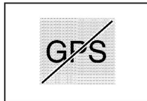
The No GPS symbol will appear, in the upper right corner of the map screen, when your vehicle is not receiving a Global Positioning System (GPS) satellite signal.
