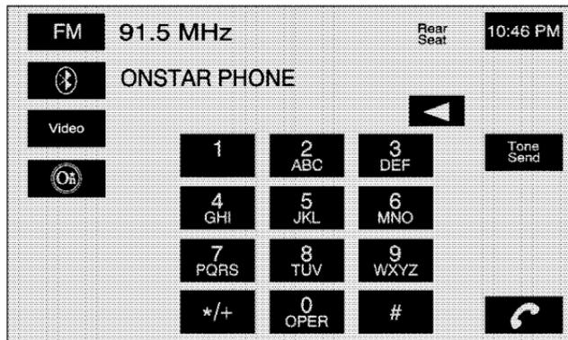
With an active OnStar® subscription with personal calling, you can make telephone calls from your vehicle, using the navigation system screen to enter the numbers.
