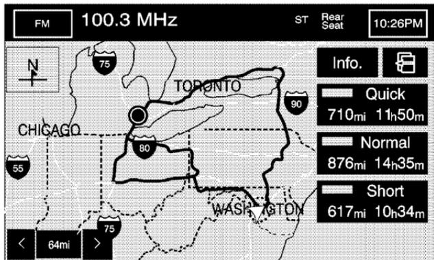
When applicable, the system will calculate up to three different versions of your current route in three different colors: Quick, Normal, and Short. The routes are shown with distance to destination and estimated travel time. The quickest route may not be the shortest, and vice versa. When an optional route is selected it is shown on the map in another color.
