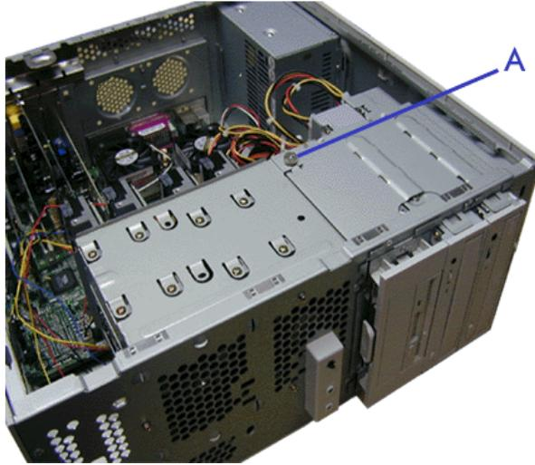
**Figure 4 - 5 : HDD Bracket Screw**
