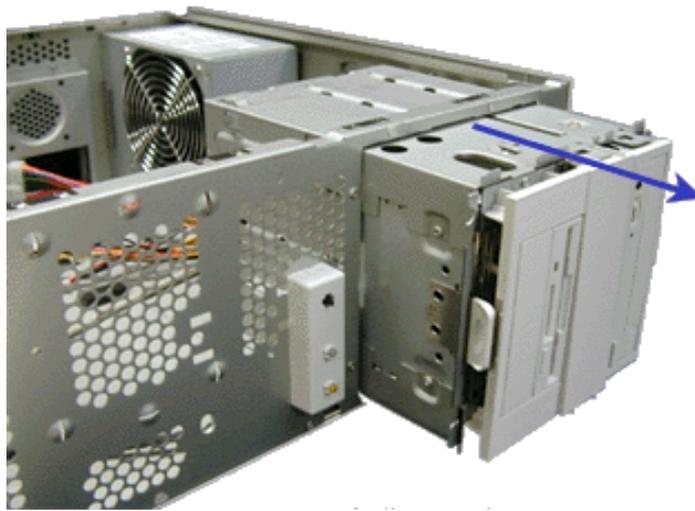
**Figure 4 - 7 : Pulling the Bracket**
