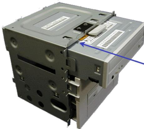
**Figure 4 - 10 : Adding a 5.25-inch Device**
