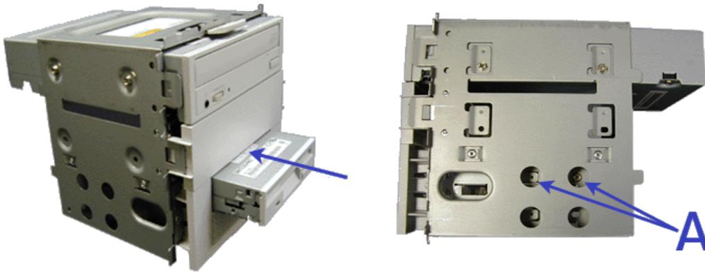
**Figure 4 - 14 : Installing a 3.5-inch Floppy Disk Drive**
