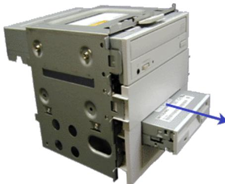
**Figure 4 - 13 : Sliding the Floppy Disk Drive out**
