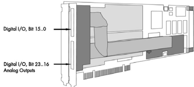
**It is not possible to use this option together with the star hub or timestamp option, because there is just space for one piggyback module on the on-board expansion slot.**
