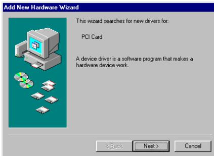
When installing the board in a Windows 98 system the Spectrum board will be recognized automatically on the next start-up. The system offers the direct installation of a driver for the board.
