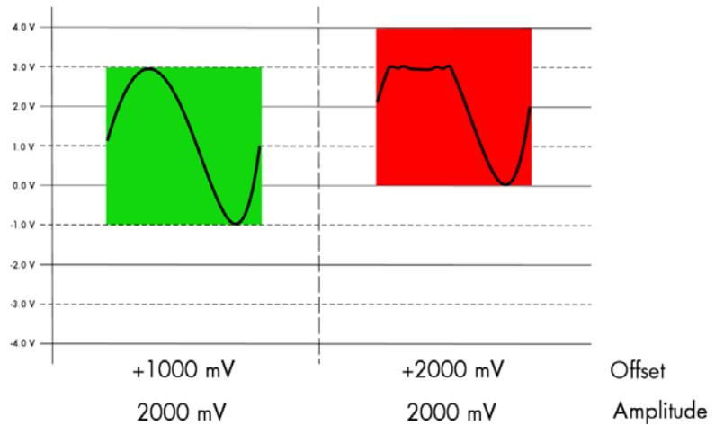
To avoid heavily distorted output signals please make sure to keep the signals in a range of  $\pm 3000$  mV.
