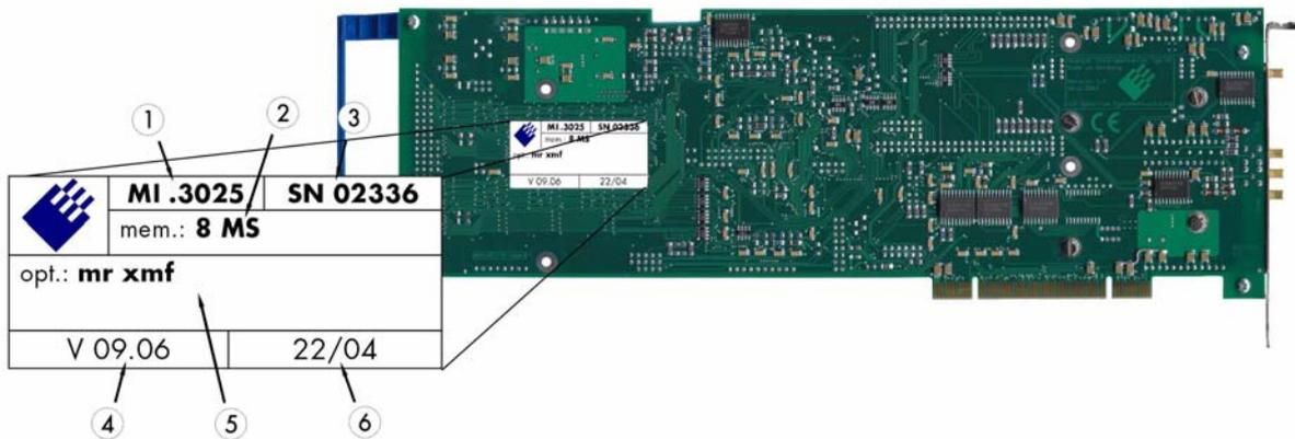
The Spectrum type plate, which consists of the following components, can be found on all of our boards.
