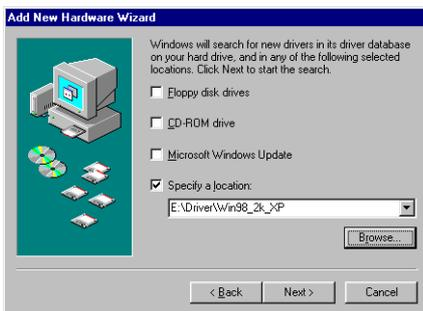
Select the CD that was delivered with the board as installation source. The driver files are located on CD in the directory \Driver\Win98\_2k\_XP. The hardware assistant shows you the exact board type that has been found like the MI.3020 in the example. Older boards (before June 2004) show „Spectrum Board“ instead.
