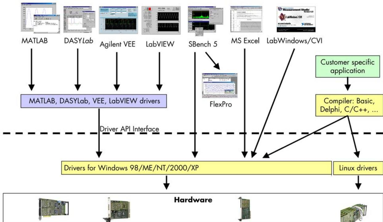
The Spectrum drivers offer you a common and fast API for using all of the board hardware features. This API is nearly the same on all operating systems. Based on this API one can write your own programs using any programming language that can access the driver API. This manual detailed describes the driver API allowing you to write your own programs.
