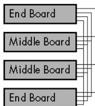
As the synchronization lines are organized as a bus topology, there is a need for termination at both ends of the bus. This is done in factory for the both end-boards. The maximum possible two middle-boards have no termination on board.
