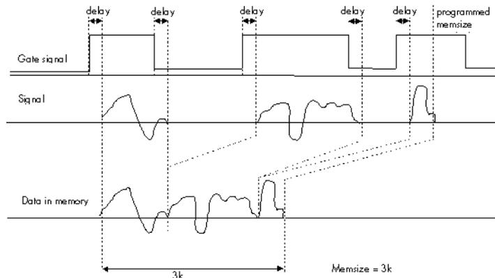
Due to the structure of the on-board memory there is another delay at the end of the gate interval.
