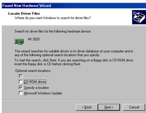
Select the CD that was delivered with the board as installation source. The driver files are located on CD in the directory `\Driver\Win98_2k_XP`.
