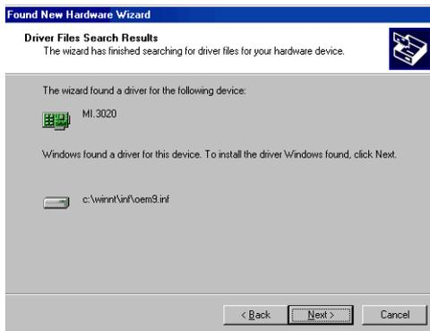
The drivers can be used directly after installation. It is not necessary to restart the system. The installed drivers are linked in the device manager.
