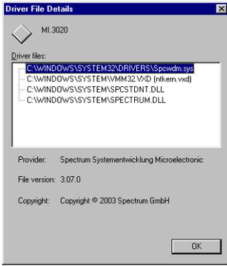
After clicking the driver info button the detailed version information of the driver is shown. In the case of a support question this information must be presented together with the board's serial number to the support team to help finding a fast solution.
