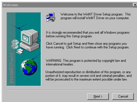
Under Windows NT the Spectrum driver must be installed manually. The driver is found on CD in the directory \Install\WinNTDrv. Please start the „Setup.exe“ program. The installation is performed totally automatically, simply click on the „Next“ button. After installation the system must be rebooted once (see picture on the right side). The driver is install to support one PCI/PXI or CompactPCI
