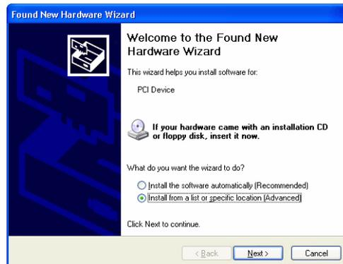
Allow Windows XP to search for the most suitable driver in a specific directory. Select the CD that was delivered with the board as installation source. The driver files are located on CD in the directory \Driver\Win98\_2k\_XP.
