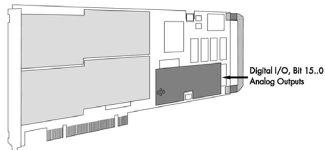
**It is not possible to use this option together with the star hub or timestamp option, because there is just space for one piggyback module on the on-board expansion slot.**
