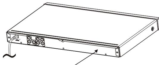
The rating plate and the safety caution are on the rear of the unit.
