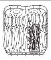
When loading the lower rack, do not load large platters or trays in the front left corner. They may prevent detergent from circulating during the wash cycle.
