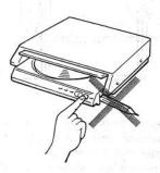
If the foreign object should be caught in this position, press the OPEN/CLOSE button immediately so that the module will move in the opposite direction.
