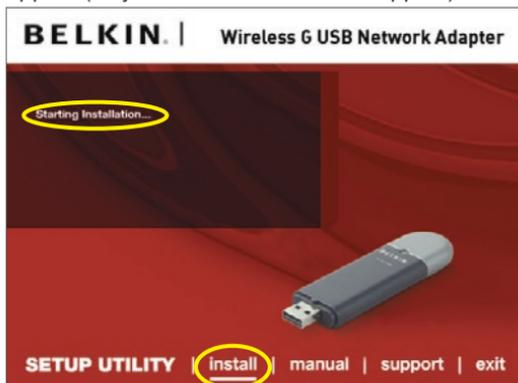
**Note:** If the Belkin Wireless Networking Utility screen does not appear within 20 seconds, access your CD-ROM by double-clicking on the “My Computer” icon; then, double-click on the CD-ROM drive into which the installation CD has been placed. Double-click on the folder named “Files”, then double-click on the icon named “setup.exe”.
