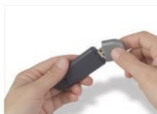
The cap snaps over the USB connector for protection.
