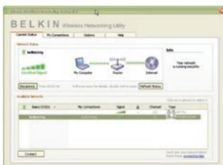
**3.2** The Wireless Networking Utility screen will appear. Select a network to connect to by selecting a network from the “Available Networks” list. Then, click “Connect”.
