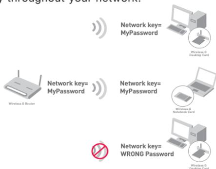
The Card cannot access the network because it uses a different network key than the one configured on the wireless router.
