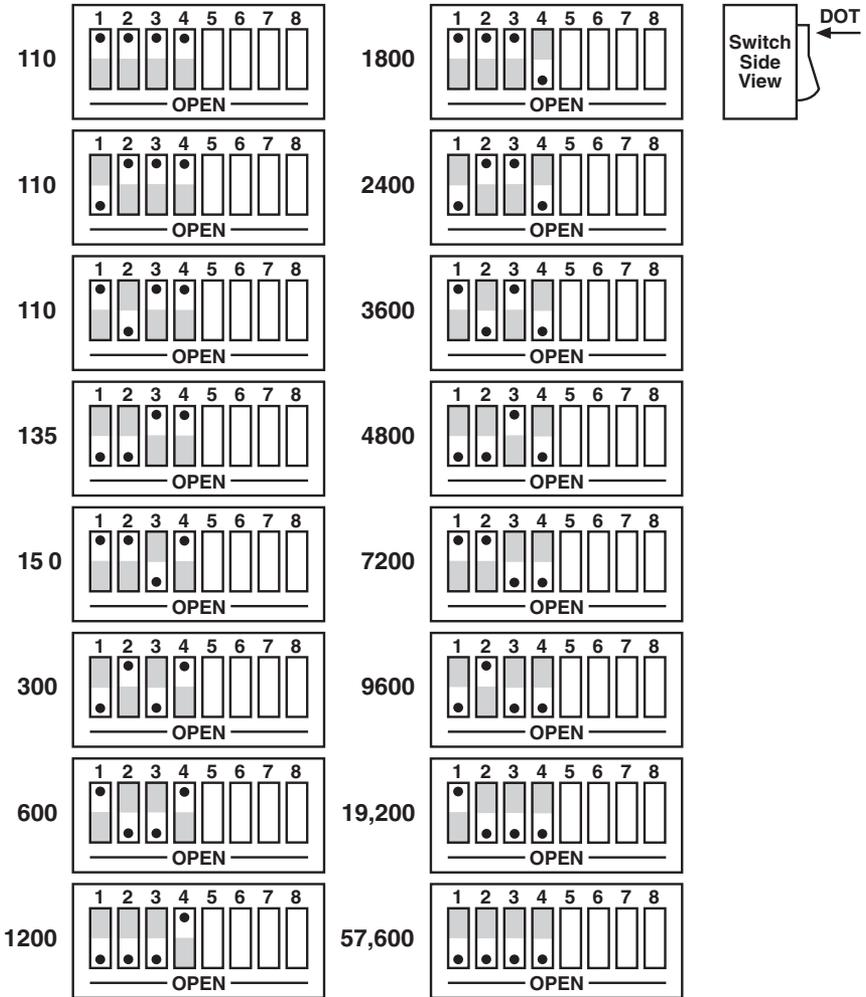
Figure 3-2. Switch SW1: Selecting the Serial Baud Rate.
