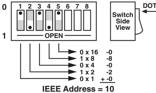
Figure 4-1. Switch SW3: Selecting the IEEE Address.
