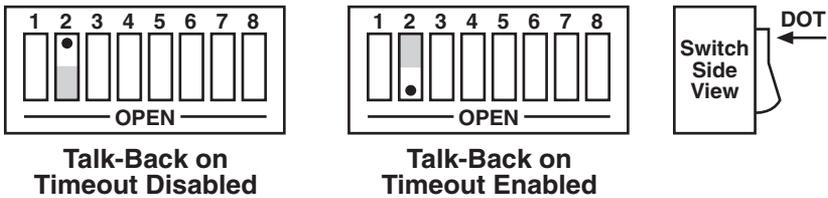
**Figure 4-3. Switch SW2: Enabling or Disabling “Talk-Back on Timeout.”**
