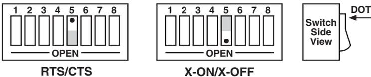
**Figure 3-7. Switch SW1: Selecting the Serial Handshake.**
