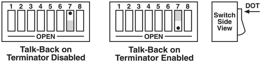
**Figure 3-12. Switch SW1: Enabling or Disabling “Talk Back on Terminator” in Controller Mode.**
