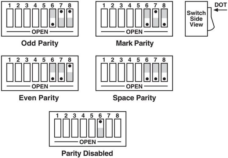
Figure 3-5. Switch SW2: Selecting the Serial Parity.
