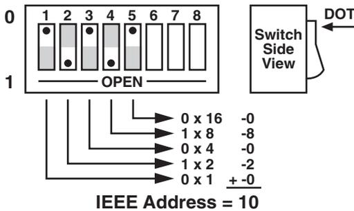
Figure 5-3. SW3 View for IEEE Address Selection.
