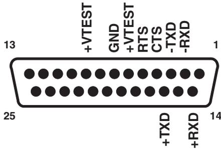
**Figure 3-16. Rear View of the Interface Converter's Serial Connector.**
