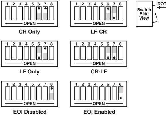
Figure 3-9. Switch SW3: Selecting the IEEE Bus Terminator.
