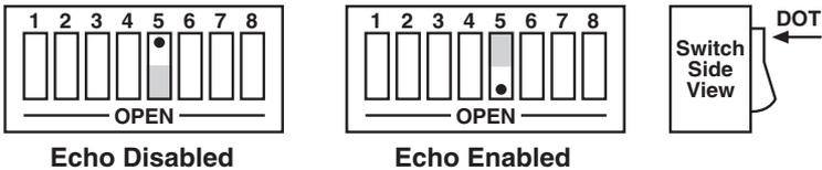
Figure 3-6. Switch SW2: Enabling or Disabling Echo.
