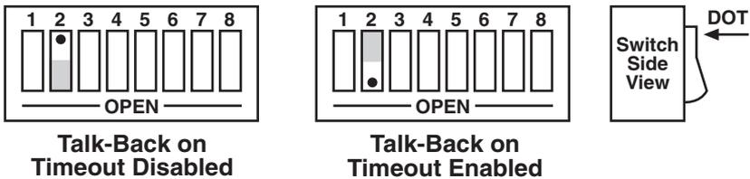
**Figure 3-13. Switch SW2: Enabling or Disabling “Talk Back on Timeout” in Controller Mode.**
