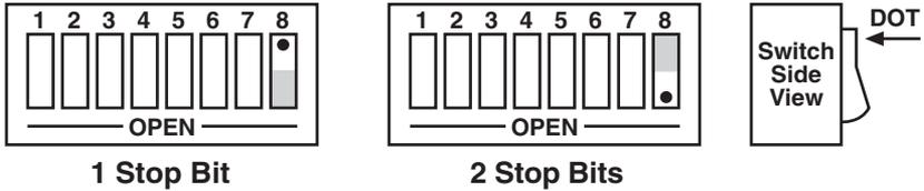
**Figure 3-4. Switch SW1: Selecting the Serial Stop Bits.**
