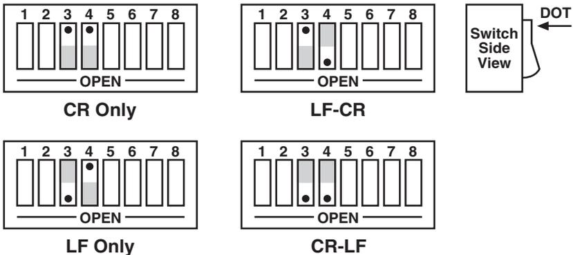
Figure 3-8. Switch SW2: Selecting the Serial Terminator.
