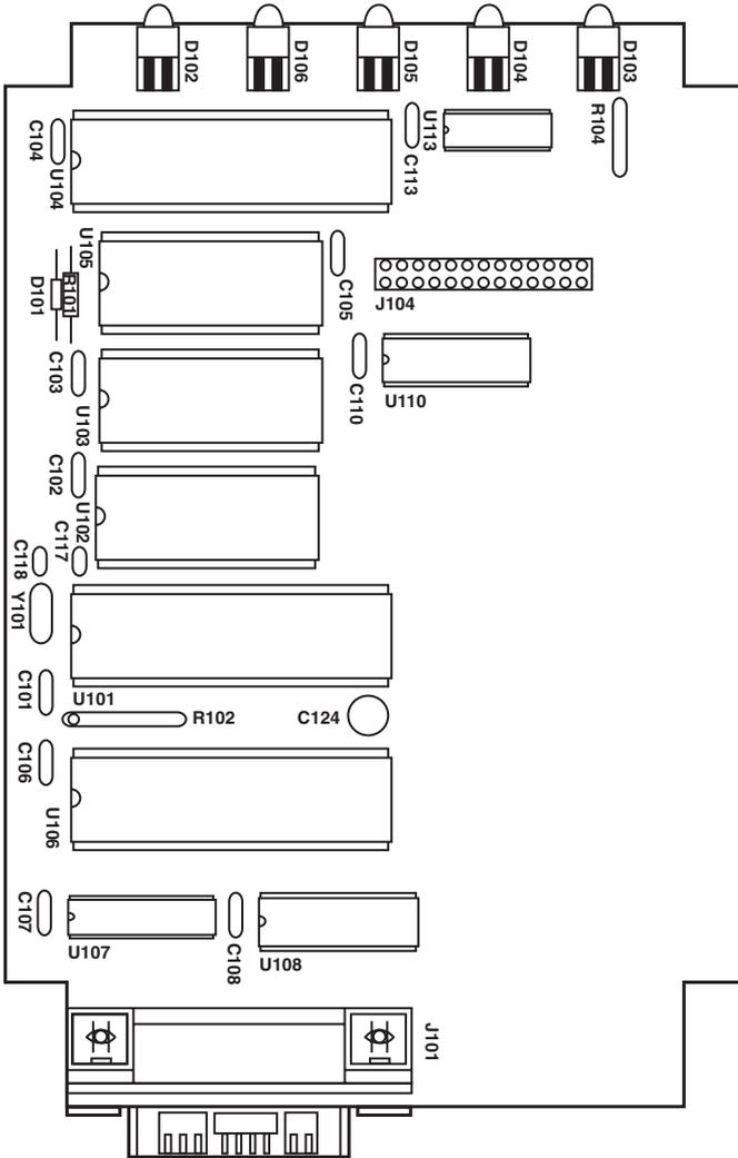
Figure 7-1. Component Layout of the Interface Converter's Motherboard.
