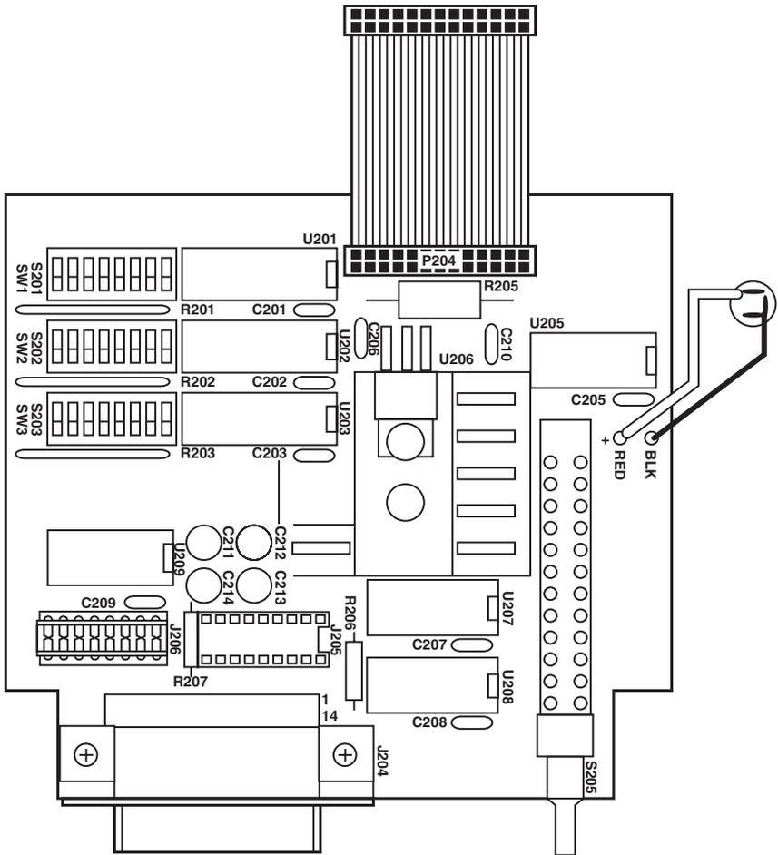
Figure 7-2. Component Layout of the Interface Converter's Serial I/O board.
