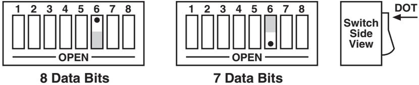
**Figure 3-3. Switch SW1: Selecting the Serial Word Length (Data Bits).**
