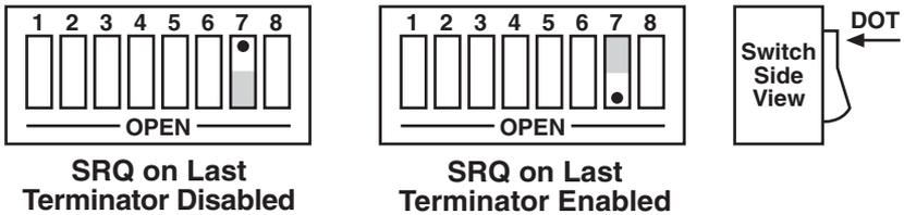
**Figure 3-14. Switch SW1: Enabling or Disabling SRQ on Last Serial Terminator in Peripheral Mode.**
