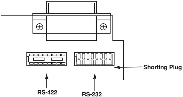
**Figure 3-15. Selecting RS-232 or RS-422 Signal Levels.**
