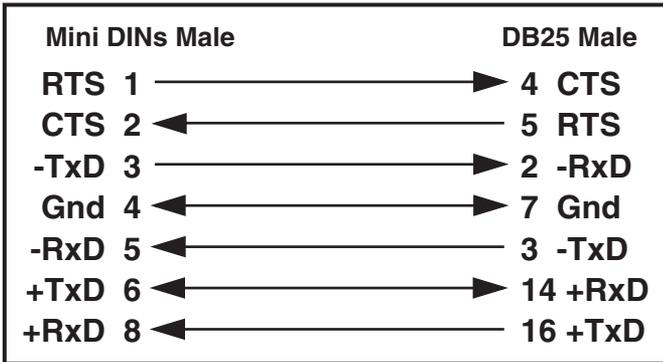
**Figure 3-17. Wiring Diagram: Macintosh to Interface Converter (RS-422).**
