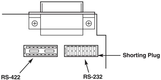
Figure 4-5. Selecting RS-232 Signal Levels.
