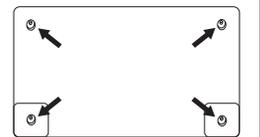
7. Ensure all four (4) screws are tight and snap caps over screw heads.
