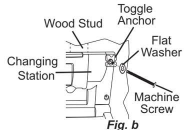
6. Align holes in changing station with drilled holes and secure top left corner of changing station to wall stud using the appropriate screw and washer. Continue to secure the three (3) remaining corners using the appropriate screws and washers as described in **Note 1** or **Note 2**.
