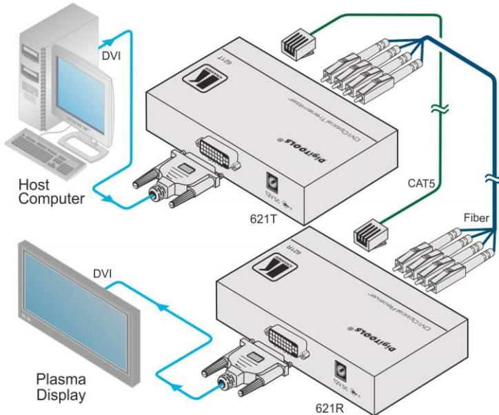
Figure 4: Connecting the 621T, 621R DVI Optical Transmitter/Receiver
