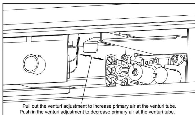
**Figure 31: Adjusting the venturi air setting.**
