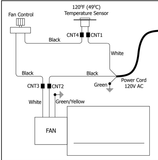
Figure 13: Fan wiring diagram.
