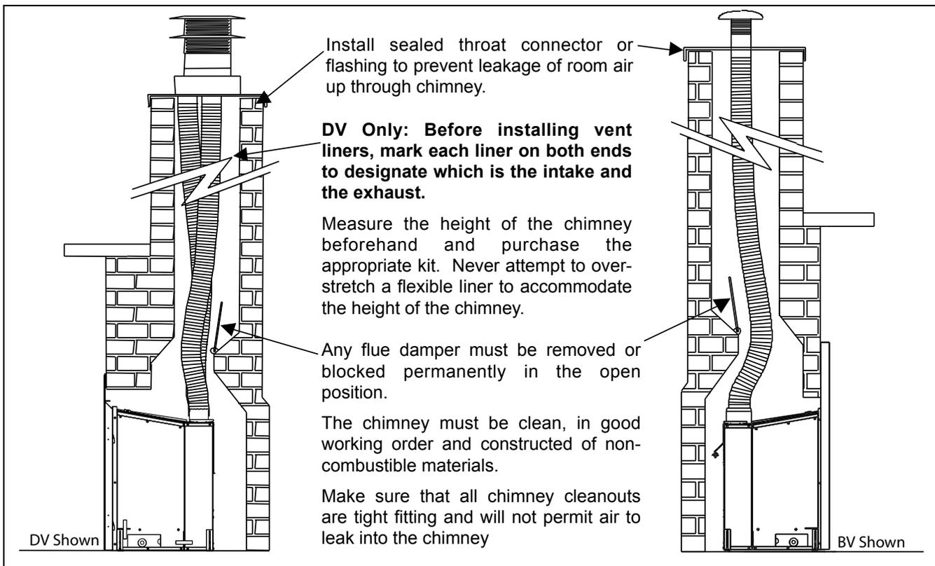
Figure 12: Installation of Sienna DV and BV.
