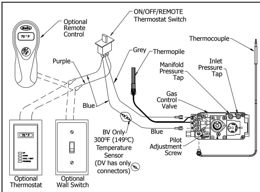
Figure 14: Wiring of a valve and thermostat.
