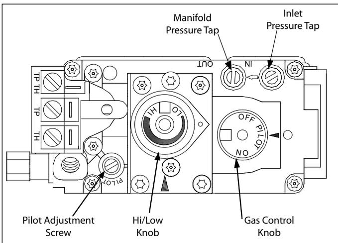
Figure 15: Fully labeled gas valve.
