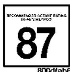
Your vehicle is designed to meet all emission regulations and provide excellent fuel economy when using high quality regular unleaded gasoline with an octane rating of 87. The use of premium gasoline is not recommended. The use of premium gasoline will provide no benefit over high quality regular gasoline, can impair engine performance and may damage the engine.
