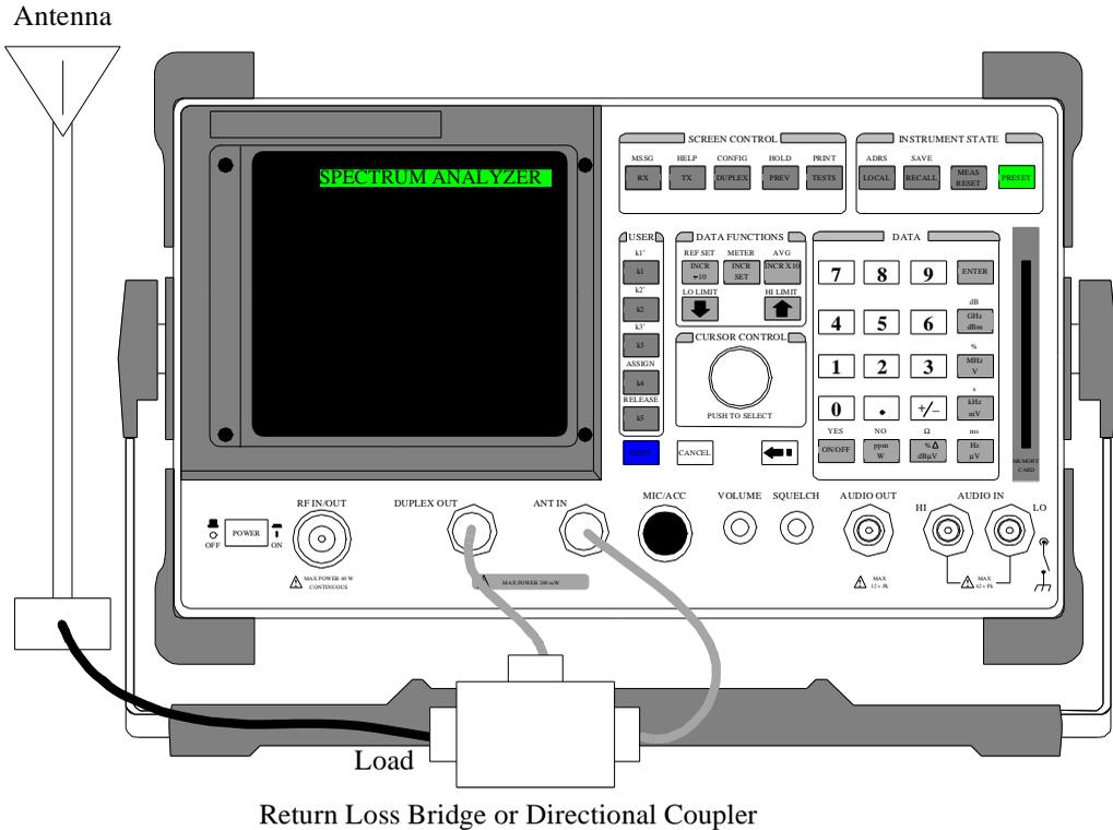
On the Test Set using the knob and data entry keys:
