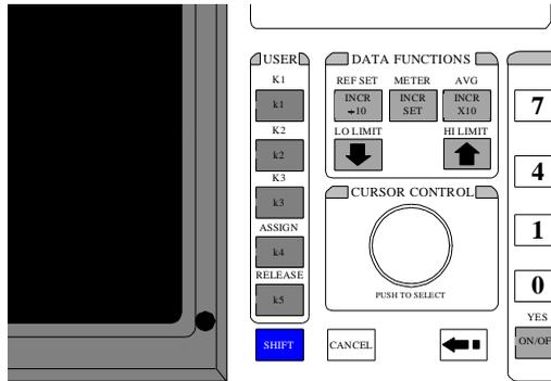
*User k1 - k5 keys* – referred to as local keys, these keys enable you to instantly enable a field for fast or repetitive access. Local keys function for fields on the screen being displayed only.
