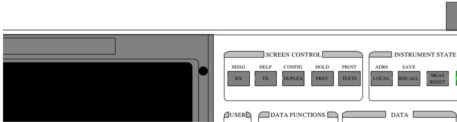
These keys are used to access several instrument control and information screens.
