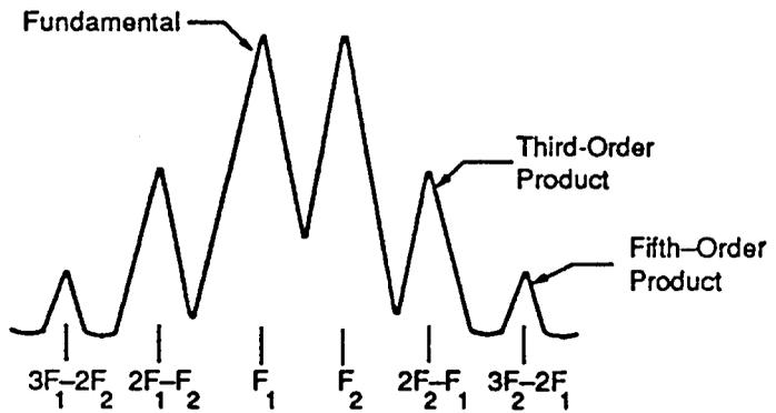
located close to the original signals at  $2F_2 - F_1$  and  $2F_1 - F_2$ , span should be reduced to as narrow as possible while still allowing the distortion products to be displayed.
