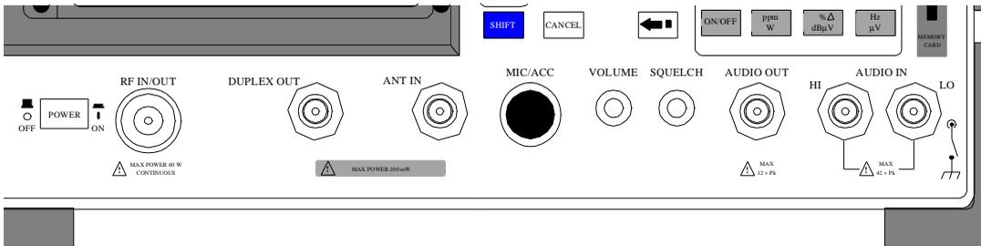
**RF IN/OUT Connector** – type-N female connector for output signals from the RF Generator, and input signals (60 Watts continuous, or 100 Watts for 10 sec/min) to the RF Analyzer. Nominal impedance is 50Ω..
