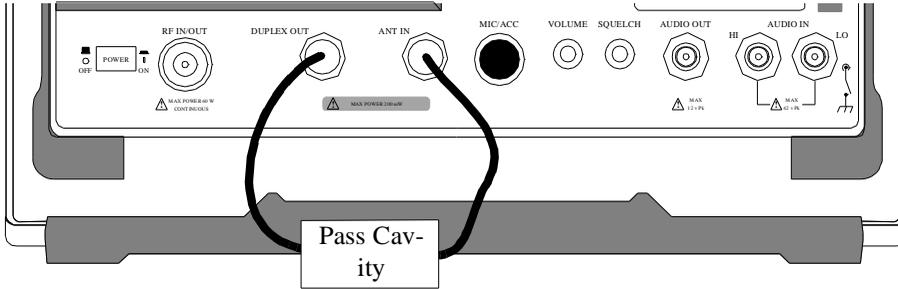
19. Adjust the tuning rod to the desired pass frequency.
