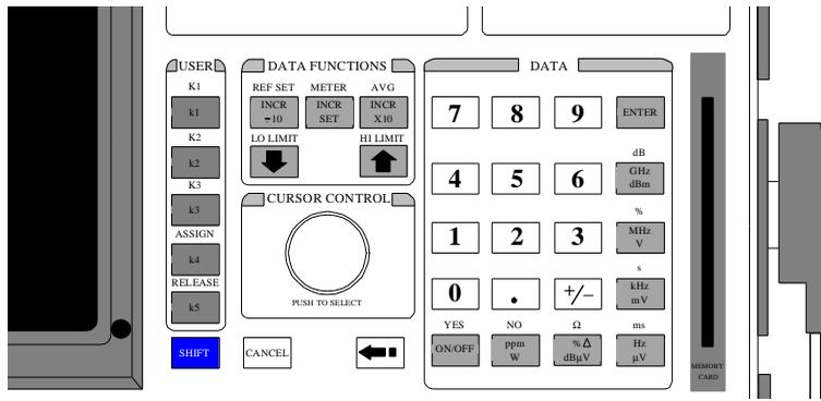
*Data Entry keys*– used to enter or change alphanumeric data (0-9, A-F, “.”, “+”, or “-”) for measurements or field entries. The EEX key is used to enter the exponent for scientific notation.
