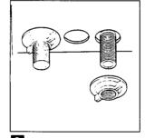
2 From underside of sink fasten faucet with plastic mounting nuts. FINGER tighten securely. DO NOT OVER TIGHTEN.
