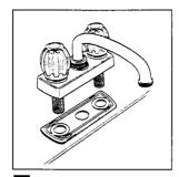
With putty plate in position, insert faucet shanks down through top of sink.
