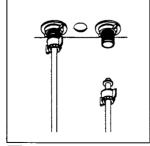
Connect hot and cold supply lines onto faucet shanks with coupling nuts. FINGER tighten securely.
