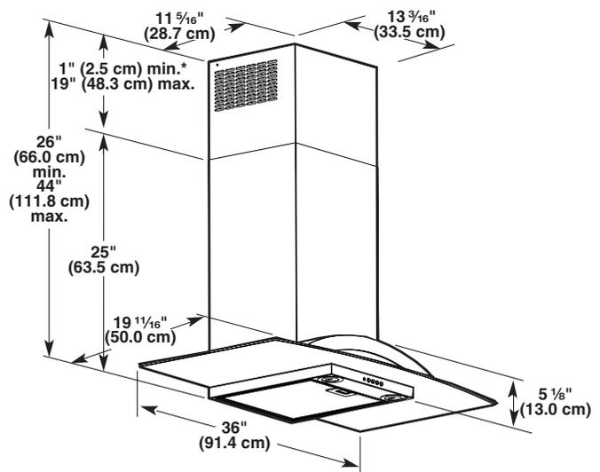
**\*IMPORTANT:** For non-vented (recirculating) installations, minimum dimension is 6" (15.2 cm).
