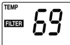
The word "FILTER" will continue flashing until the filter counter is reset back to zero.
