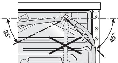
2. Connect the hose with the straight connection to a water tap with a screw thread R 3/4 (inches)
