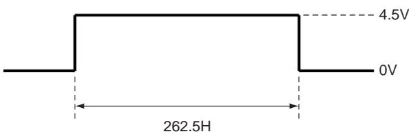
The amplitude level is the representative value when terminated with 10kΩ.
