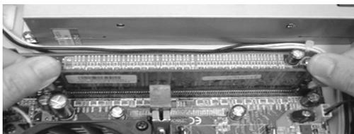
**Step 3:** Press the latches into the notches of the RAM module.
