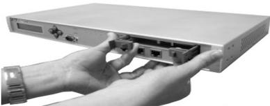
**Step 3:** Remove the mobile rack straight and smooth.
