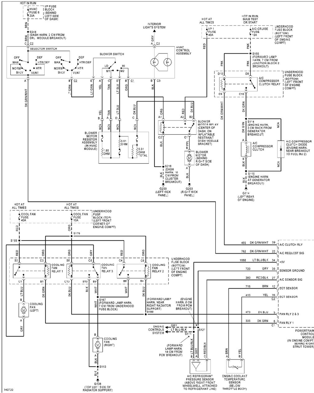
Fig. 6: Manual A/C-Heater System Wiring Diagram (2001 Camaro & Firebird With 3.8L Engine)
