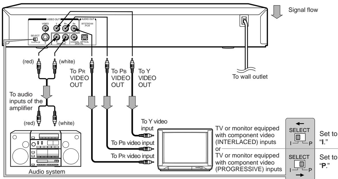
■ **Switching the output signal (interlaced/progressive) using the remote control (only when the SELECT (I/P) switch is set to "P")**
