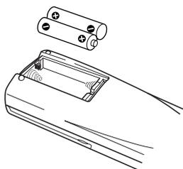
Make sure to match the + and – on the batteries to the marks inside the battery compartment.
