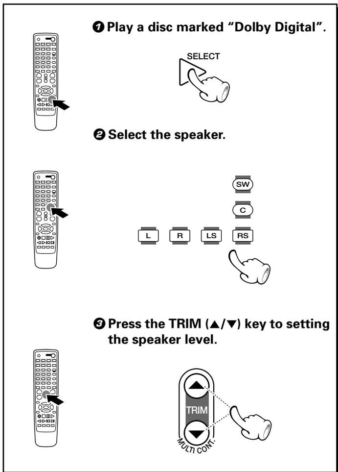
Speaker level adjustment can be performed by pressing the keys L, R, SL, SR, C and SW.
