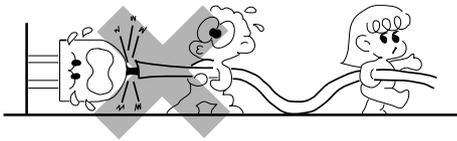
**3. CAUTION – Polarization** – This appliance may be equipped with a polarized alternating-current line plug (a plug having one blade wider than the other). This plug will fit into the power outlet only one way. This is a safety feature. If you are unable to insert the plug fully into the outlet, try reversing the plug. If the plug should still fail to fit, contact your electrician to replace your obsolete outlet. Do not defeat the safety purpose of the polarized plug.
