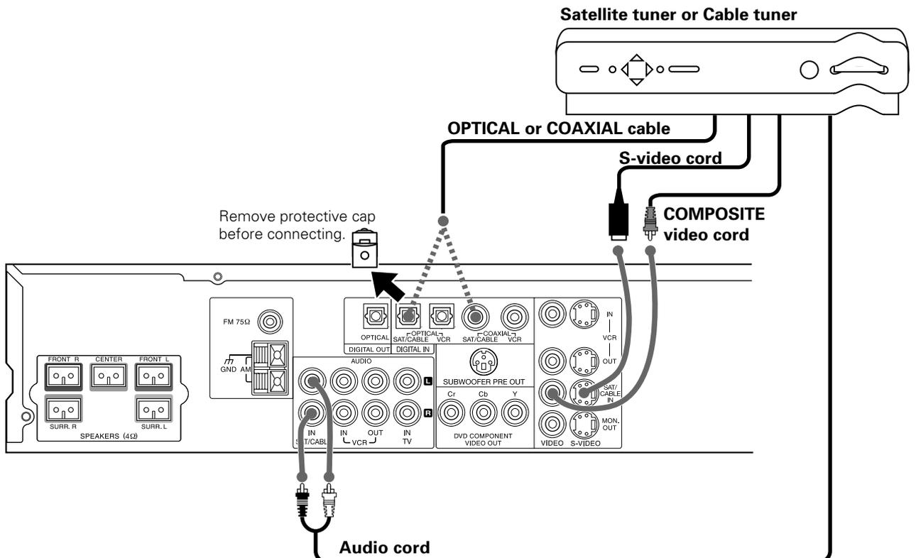
Connect the OPTICAL or the COAXIAL cable, depending on the digital output of the satellite tuner.
