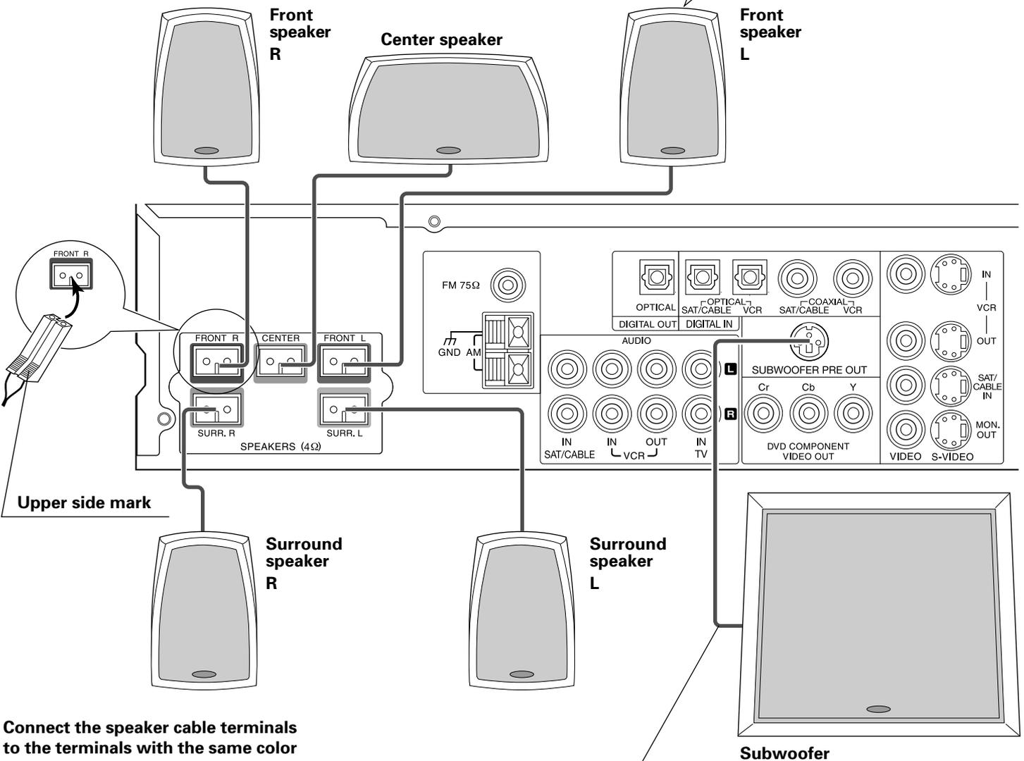
Connect the speaker cable terminals to the terminals with the same color at the speaker terminal panel on the main unit. Connect matching the color of the speaker terminal (+ side) and the color of the speaker cable tube.
