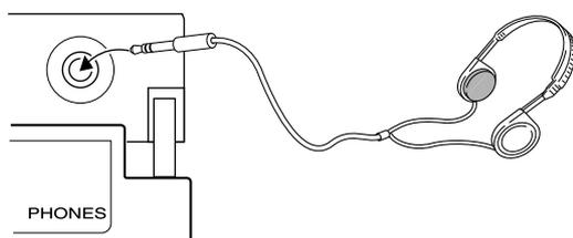
This unit offers various surround modes, but it switches automatically to stereo mode when headphones are connected.
