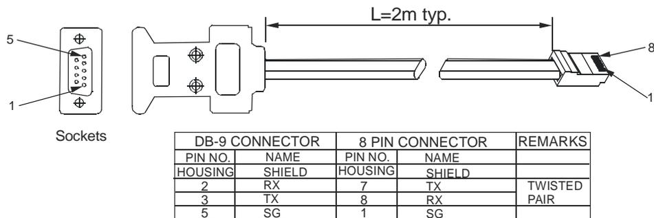
Fig.7-3: RS232 cable with DB9 connector (P/N: GEN/232-9)
