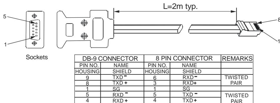
Fig.7-4: RS485 cable with DB9 connector (P/N: GEN/485-9)
