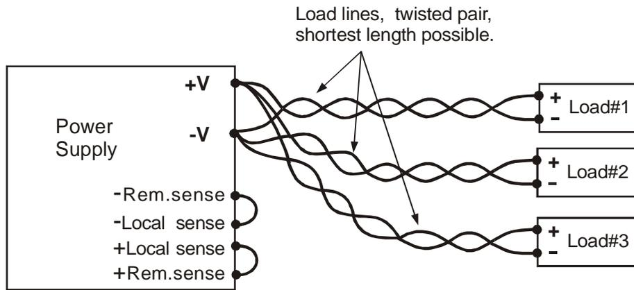
Fig.3-12: Multiple loads connection, radial distribution, local sense
