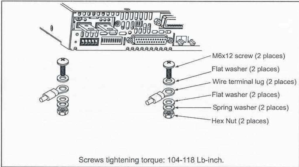
Fig. 3-5: Load wires connection , 6V to 60V models.
