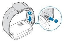
Note: If you replace the strap on your Gear 2™ with another strap not manufactured by Samsung, please use a strap with a standard 22mm spring bar pin, and refer to the manufacturer's instructions to properly attach the band.
