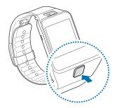
2. Press and hold the Power button, and then tap Power off to turn off the Gear 2™.
