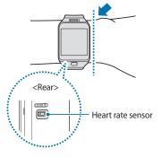
Important! Remove the protective plastic from the heart rate measurement sensor before taking measurements.
