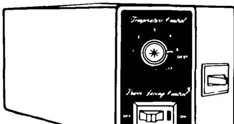
1. Before freezing large quantities of food, turn Temperature Control to highest setting and let freezer operate for several hours. **After loading all food items, return Temperature Control to the usual setting.**
