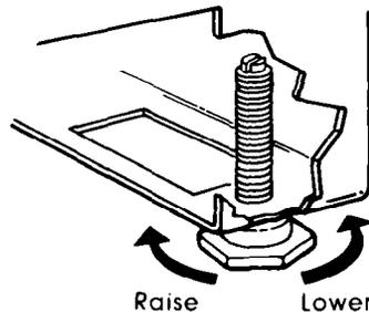
1. Keep the 4 bolts that hold refrigerator in shipping crate. They are the levelling legs.
