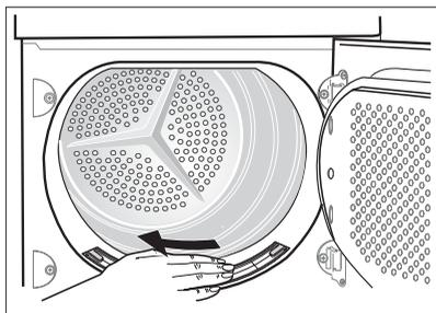
3. After a period of time, a patina due to detergent residue on laundry forms on the filters. When this occurs, clean the filters with warm water using a brush. Remove the filter from the door pulling it out. It can be positioned with the tooth facing to the left or to the right. After cleaning do not forget to put it back.
